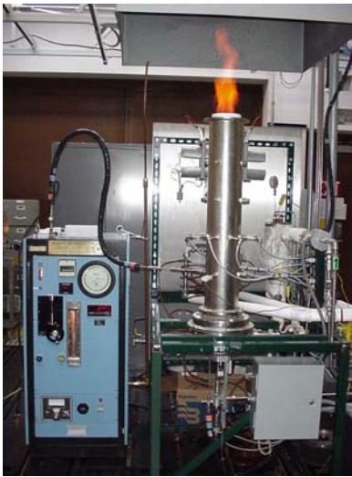
Figure 3: WSR Inside Housing Section, Attached to PFR Stack, Burning Premixed Methane-Air.
