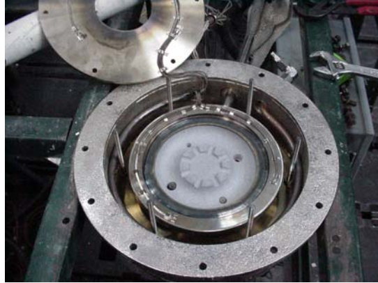
Figure 5: Jet Ring Atop Bottom Half of Silicon Carbide Reactor, Mounted in Housing.
