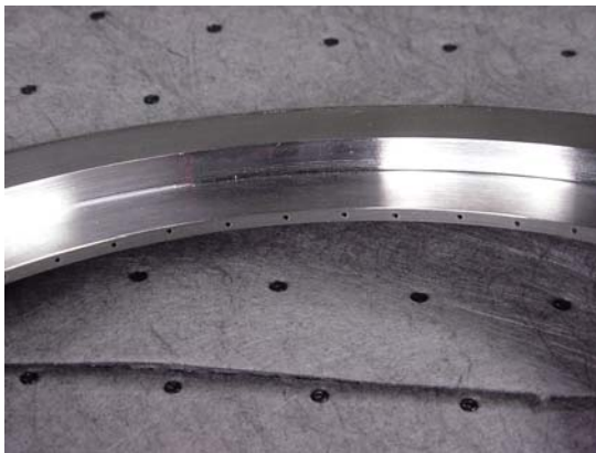
Figure 4: Inconel Jet Ring Containing 48 Fuel-Air Jets.
