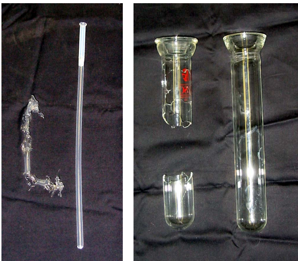
Fig. 18. Before And After Pictures of a 10 mm o.d. Teflon™-FEP tube (left picture) and a 45 mm o.d. heavy wall Pyrex™ waste trap (right picture), destroyed by about 0.5 mmol of typical polyazides.
