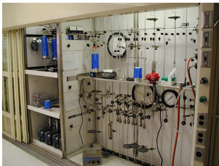
Fig. 6. One Of The Six Walk-In Fume Hoods of the New USC Laboratory Each fume hood is equipped with a custom-built stainless-steel/Teflon™ and glass vacuum line.
