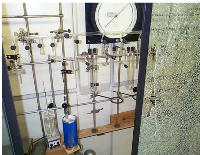
Fig. 8. Typical Damage Caused by an HN_3 Explosion One trap of the glass line is missing, and parts of it have penetrated the safety glass of the door.
