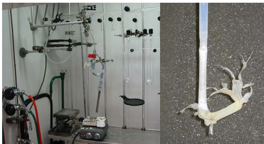
Fig. 13. Typical Damage Caused by the Explosions of About 0.5 mmol of N_5^+P(N_3)_6^- In the left picture, the explosion destroyed the heavy ceramic plate of a stirring plate. The right picture shows the close-up of an exploded Teflon™ reaction tube.
