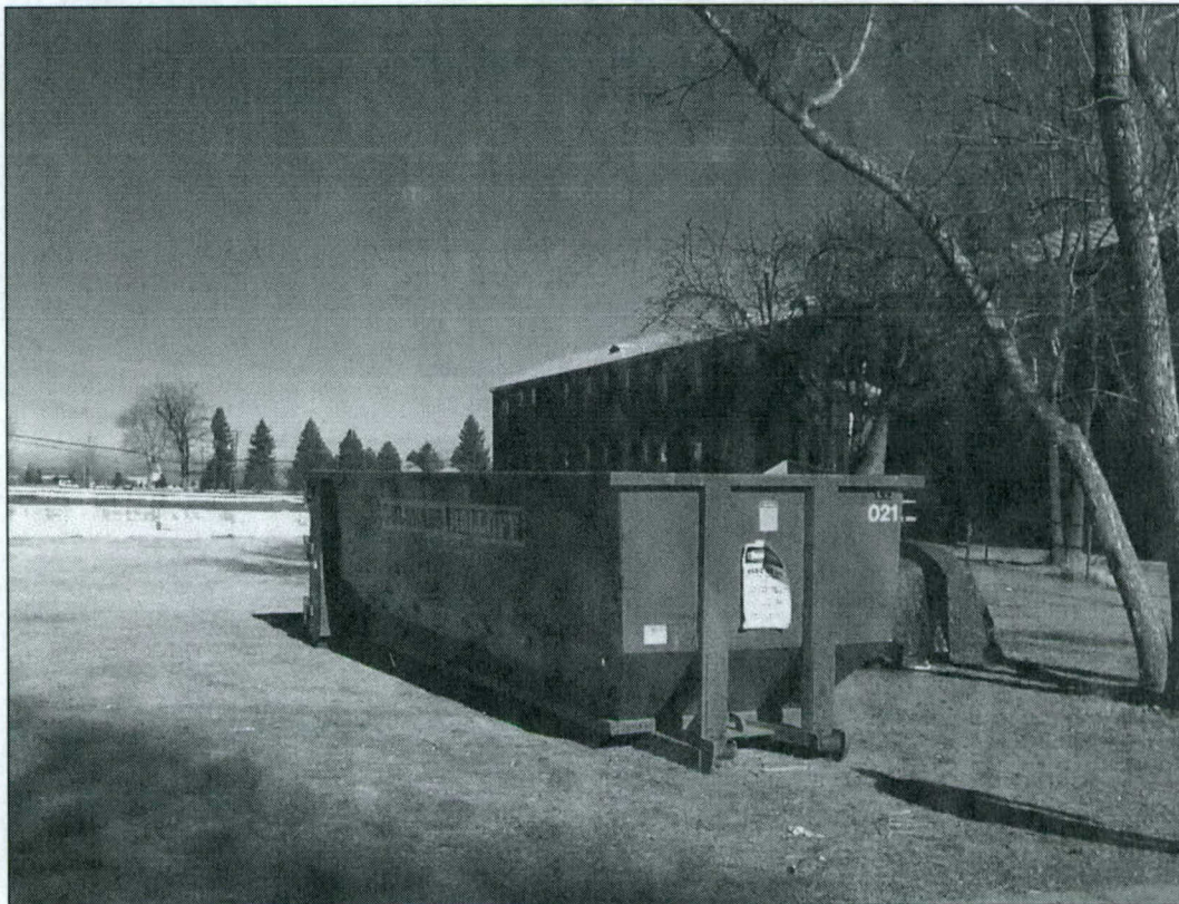
Figure 5. Forty cubic yard roll-off waste container.
