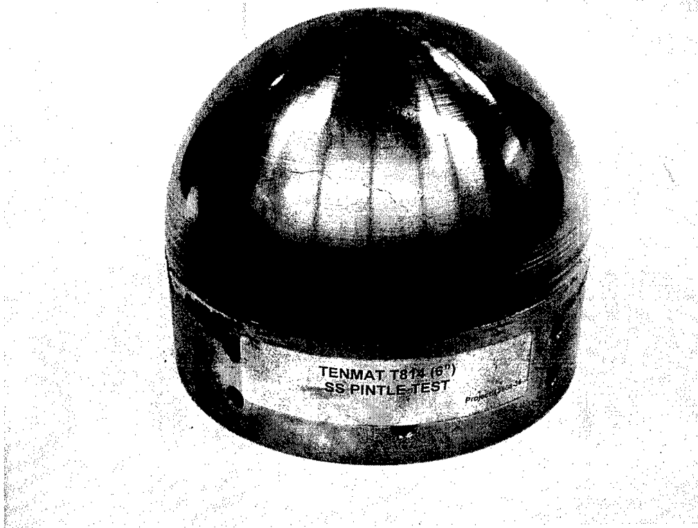
Figure D7. Overview of 6" Tenmat T814 pintle. Note transferred lubricant material on side of pintle contact surface.
