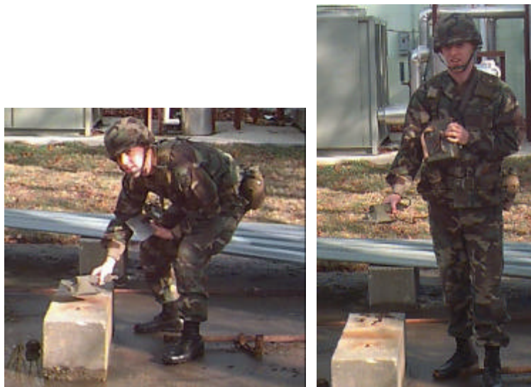
Figure 7-E: The proper use of the alpha probe is shown on the left and the improper use is on the right.
