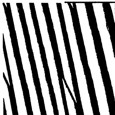
Fig. 3. Ag/Cu striped nanostructure grown on Cu(775). Cu(111) terraces alternate with Ag covered [773] facets (inset) (200nm, 1.5 V, image derivative along the horizontal direction).
