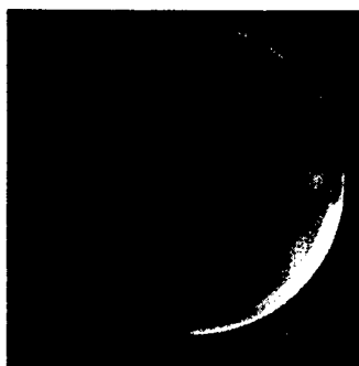
Fig. 1a A typical emission pattern of a multiwalled CNT, at 1.6 \cdot 10^{-6} mbar N_2 , 2.1 kV extraction voltage, and pre-heated at 1100 °C.
