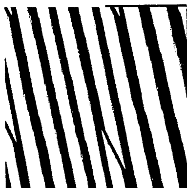
Fig. 3. Ag/Cu striped nanostructure grown on Cu(775). Cu(111) terraces alternate with Ag covered [773] facets (inset) (200nm, 1.5 V, image derivate along the horizontal direction).
