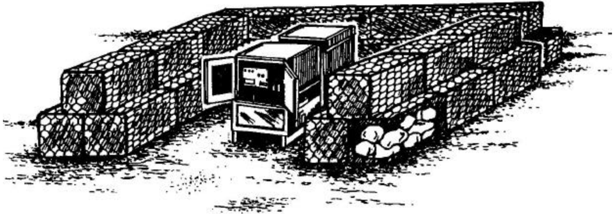
Figure 34. Rock Filled Gabion Walls.
