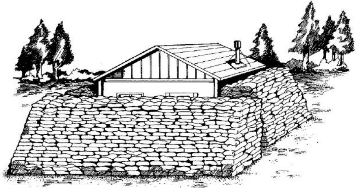
Figure 19. Sandbags Help Support Roof Covering.
