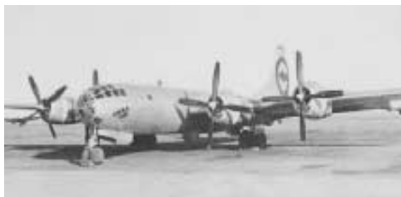
The Enola Gay was one of 15 B-29s modified specifically for the highly secret atomic bomb missions. These airplanes were outfitted with new engines and propellers and faster-acting pneumatic bomb bay doors.
