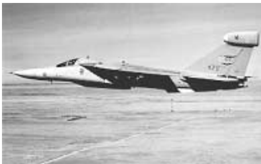
The EF-111 Raven was used to jam Libyan search radar and provide electronic countermeasures against any surface-to-air threats.
