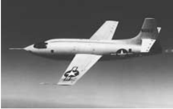
The Glamorous Glennis piloted by Capt Chuck Yeager, was the first aircraft to break the sound barrier.
