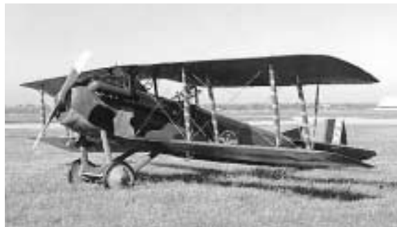
Bullard flew the Spad XVI, a French-designed and -built fast two-seat reconnaissance-type aircraft developed from the Spad VII. At the time of its entry into service (1916), it was one of the fastest and most maneuverable two-seaters in combat.
