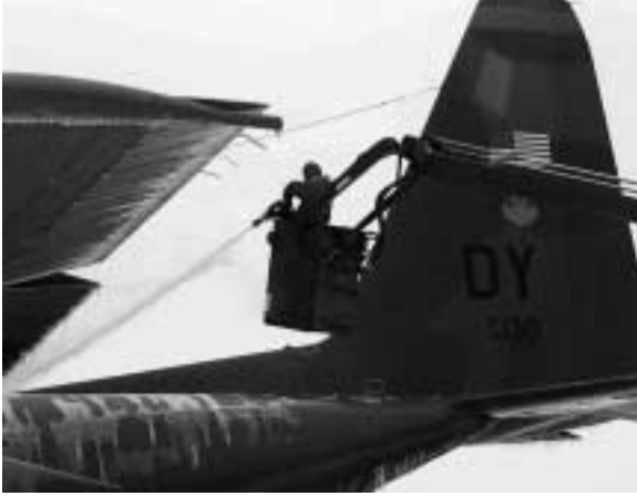
C-130s, like this one being deiced before a mission in the Balkans, were the backbone of Operation Provide Promise.
