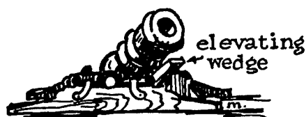
FIGURE 36—ENGLISH MORTAR ON ELEVATING BED (1740).
