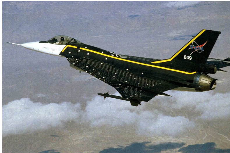
Figure 1. F-16XL-1 airplane in flight with missiles, tufts, modified flow-visualization paint-scheme and video targets at NASA-Dryden.
