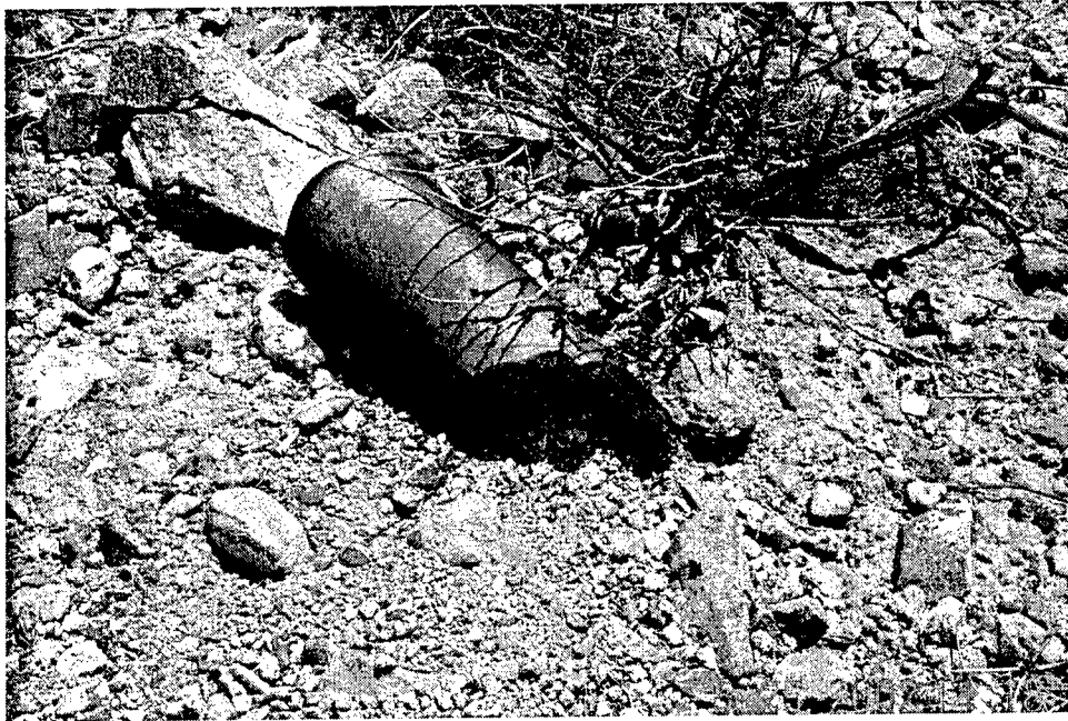
Figure 2-10. Photograph of low-order 2.75-in. rocket warhead, Dona Ana Range, Fort Bliss, New Mexico
