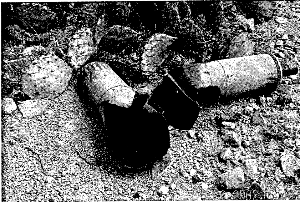
Figure 2-13. Photo of two low-order recoilless rifle rounds at Dona Ana Range, Fort Bliss, New Mexico
