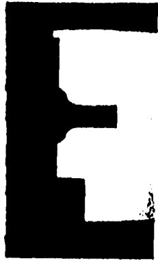
FIGURE 2 A typical digitized image of the deformed impact specimen. The lower body is the fiducial, a structure with known dimensions which gives longitudinal and lateral dimensions.
