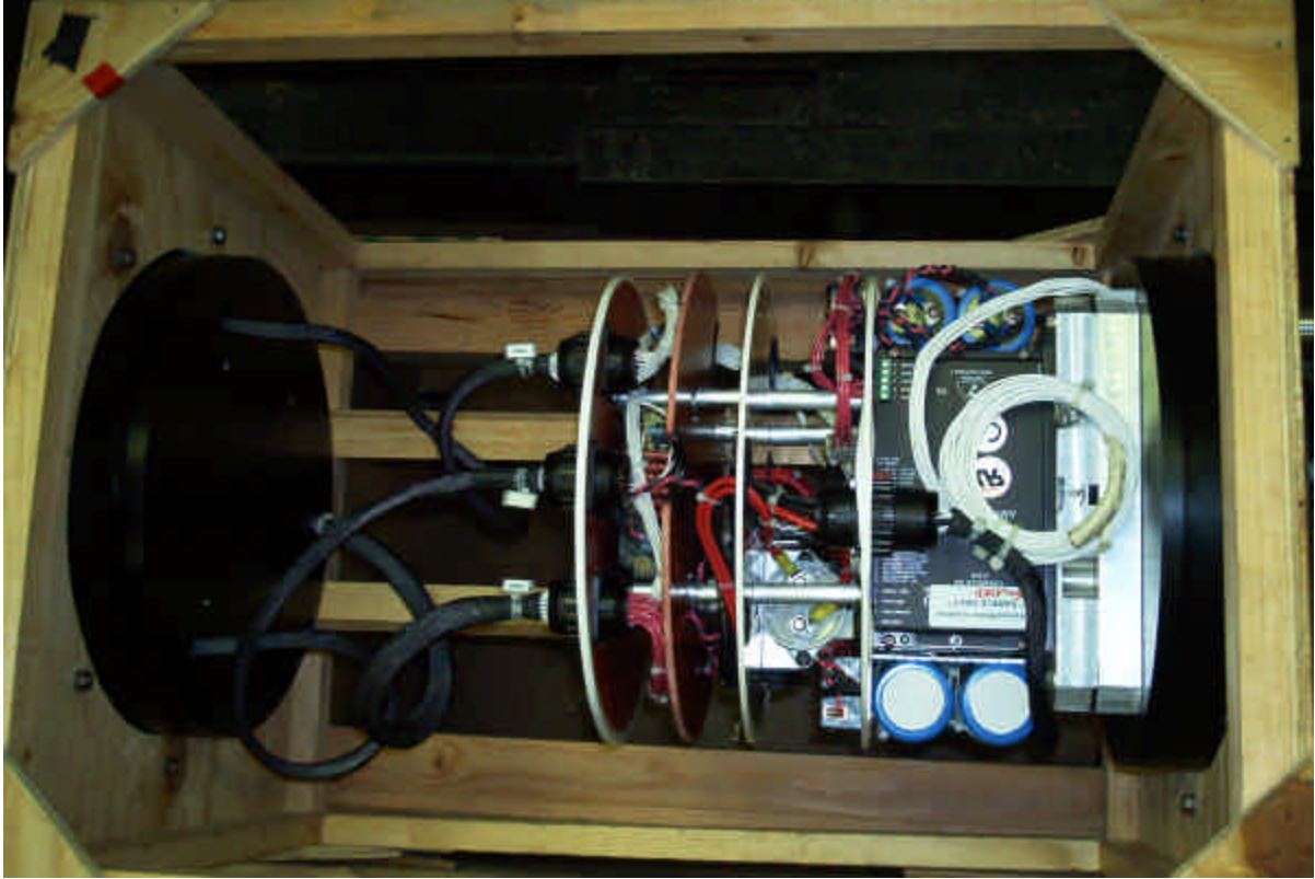
Figure MED-71: Top View of PV#6 Thruster Controller Electronics.
