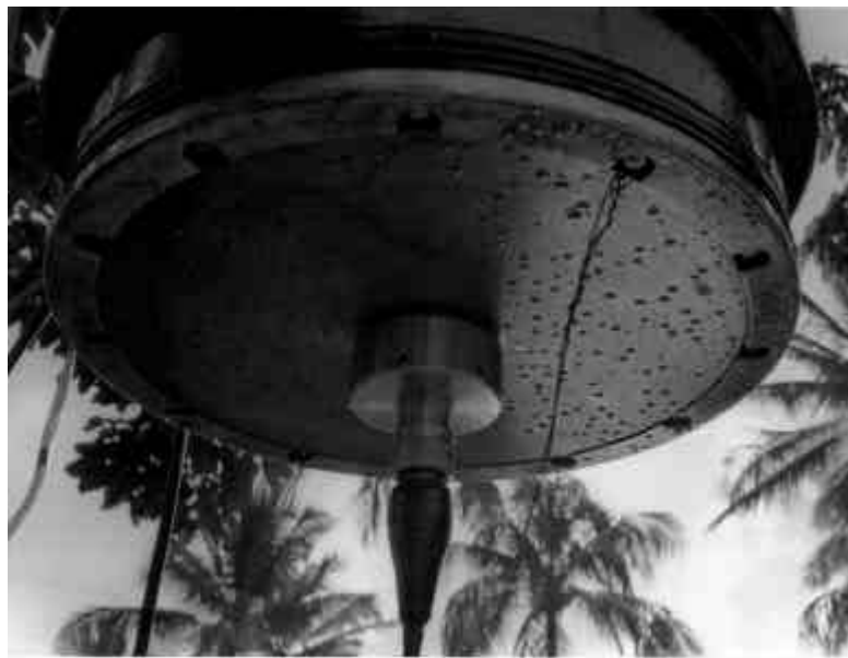
Figure MAF-63. Photograph of the Pressure Chamber End-cap and the Connector
