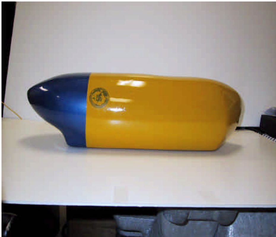
Figure MED-3: 1:12 Scale Model Plug for Tank Testing.
