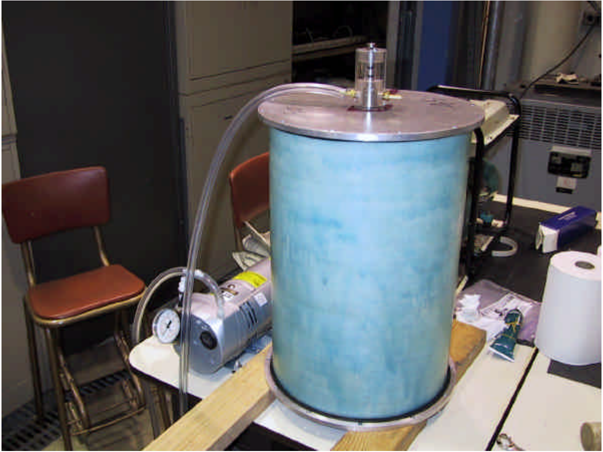
Figure MED-12 - Vacuum Hold Test and Lid Installation
