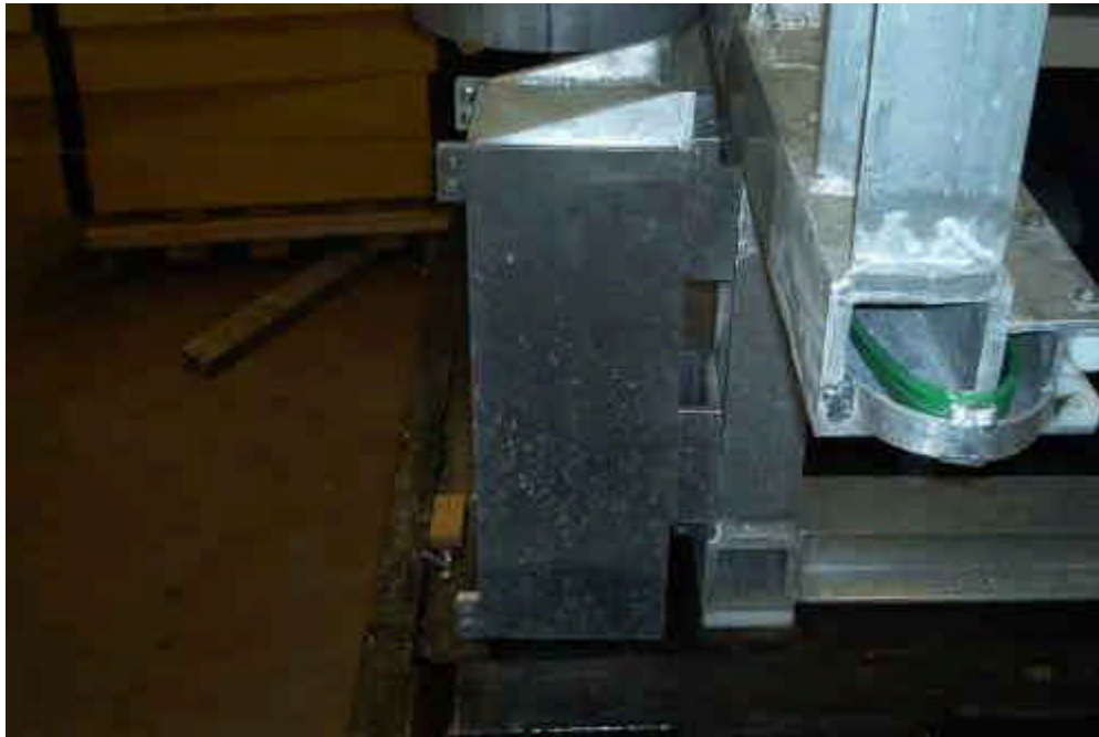
Figure MED-31: Starboard Forward Ballast Mount on Forward Corner of Frame.
