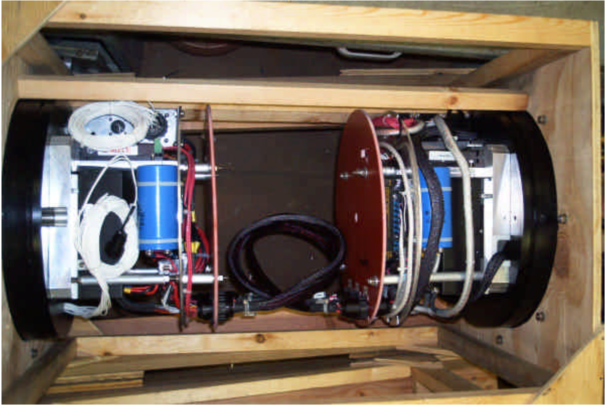
Figure MED-69: Top View of PV#5 Thruster Controller Electronics.
