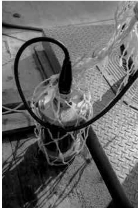
Figure MAF-62. Photograph of the Scaled Pressure Vessel and the Connector
