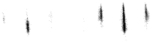
Fig. 3. RHEED streaks acquired on as-deposited (left) and after annealing at 250 °C (right) 8-Å-thick Co layers. Before annealing streaks are blurred, but single and correspond to the lattice constant 2.72 Å. After annealing they are split revealing the lattice parameter 2.59 Å and 2.83 Å for outer and inner, respectively.
