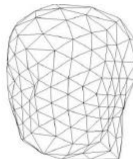
Fig. 2. Phase one - the surface S' obtained after the expansion and uniform re-sampling of the icosahedron of previous Fig. 1.
