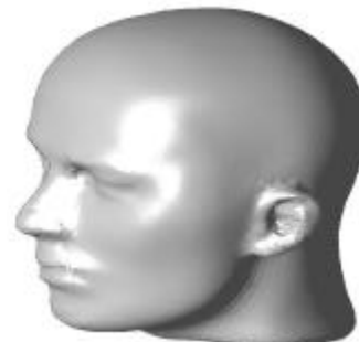
Fig. 4. Phase three - the final surface S''' at the end of the reconstruction process. This surface is obtained by smoothing the surface S'' of previous Fig. 3. Here, for rendering purposes, the triangles of the mesh surface S''' were uniformly colored and a spot light was added to the scene.
