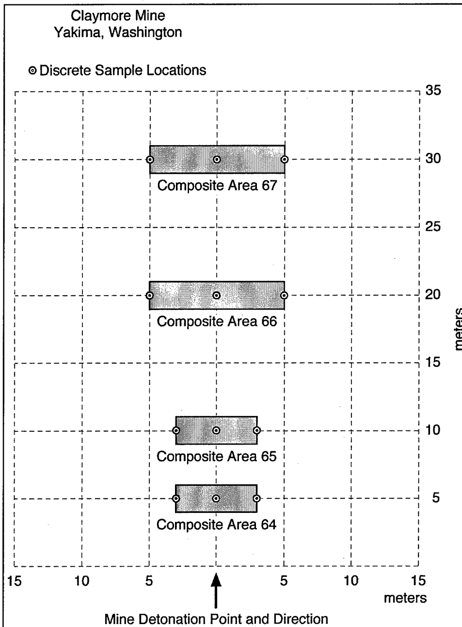
Figure 14. Soil sampling locations in front of location where Claymore mine had been detonated at Yakima Training Center
