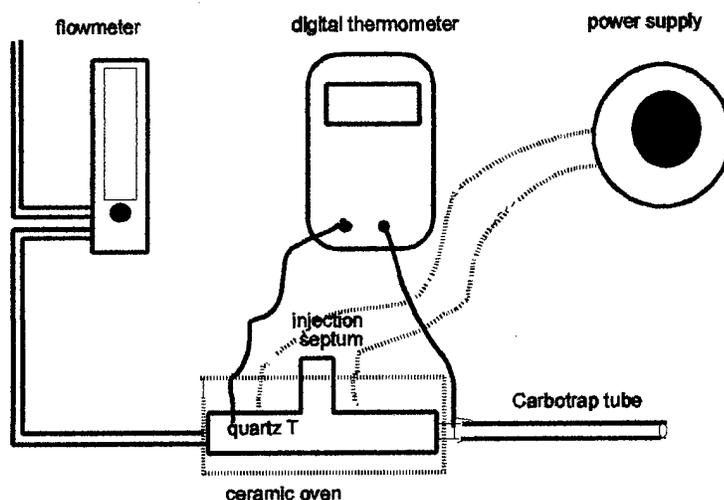
**Figure 4.2.1** Calibration device for introducing the internal standard and system monitoring compounds into the TD/GC/MS sampling tubes. Samples are "pushed" onto the trap by a helium carrier gas flow from the flowmeter, but beyond that, sorbed in an analogous manner to field samples.
