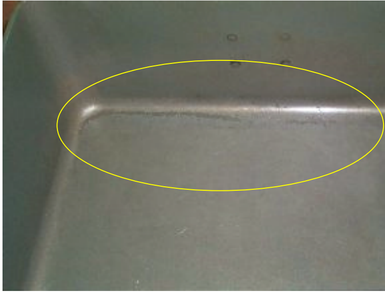
Figure 30. Teflon® peeling away at the corners and fillets
