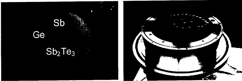
Figure 6. Left panel: Target used for co-sputtering, consisting of Ge, Sb and Sb 2 Te 3 segments. Right panel: Magnet configuration of the rotating-magnetron cathode used for co-sputtering.
