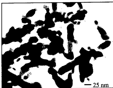
Figure 4 : TEM image of \text{Mn}_{1.7}\text{Fe}_{1.3}\text{O}_4
