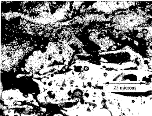
Figure 6. Optical micrographs of WC/12Co nano-coating samples, comparing microstructures (etched condition) of (a) HVOF coating, (b) N 2 /H 2 -plasma coating, and (c) HVOF overlay coating on N 2 /H 2 -plasma coating. Note uniform distribution (speckled appearance) of fine WC particles in (a), and the absence of WC particles in (b), due to extensive decarburization in the N 2 /H 2 -plasma coating.
