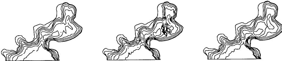
Figure 9: Depth contours for bilinear interpolation using 3 depth points (left), Taylor series interpolation using 5 depth points with 2 sets (middle) and inverse power interpolation using 4 depth points with m=4 (right)
