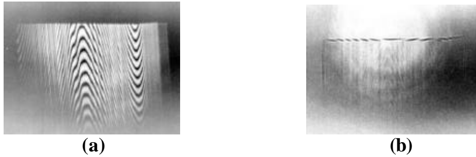
Fig.5. The interference pattern obtained in the beam reflected by the cover glass (a) and the corresponding OV street in the transmitted beam (b).
