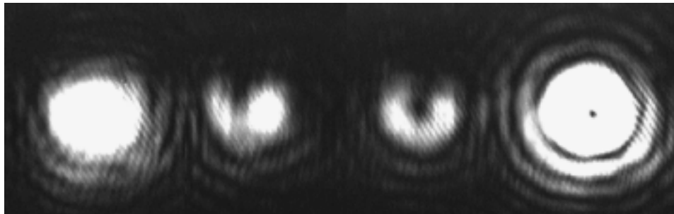
Fig. 6. Diffraction orders, from left to right: zero, subharmonic 1/3 , subharmonic 2/3 , first.
