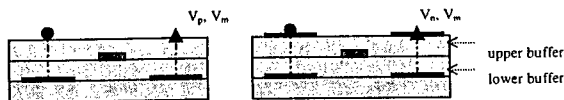
Fig.1 Transverse structures: a. single bottom transverse electrodes (SBT). b. double transverse electrodes (DT)
