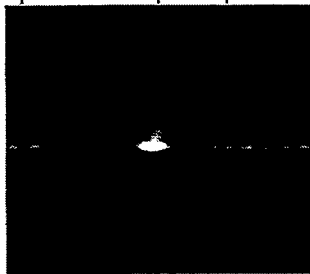
Figure 2: Outcoupled 1064 nm beam of a 5 \mu m wide photobleached waveguide. Scattered light is guided in the bleached layer on both sides of the channel waveguide.
