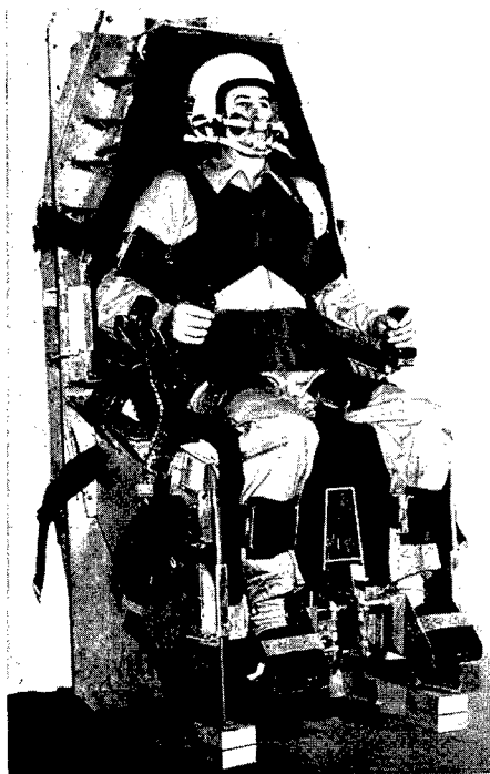
Fig. 2. Over-all view of restraint system.
