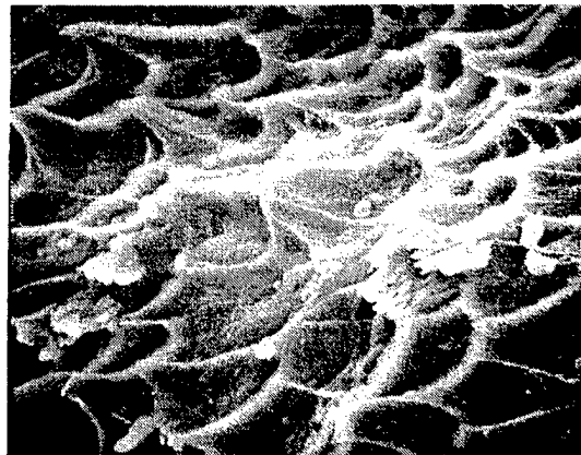
Photo 9. SEM photo showing ductile area of the titanium material at 2500X magnification
