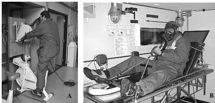
Figure 2: Photographs of two types of prebreathe exercises used to augment nitrogen washout. Figure 2a shows the dual arm/leg ergometry used in Phase II. Figure 2b shows Phase IV prebreathe exercises.
