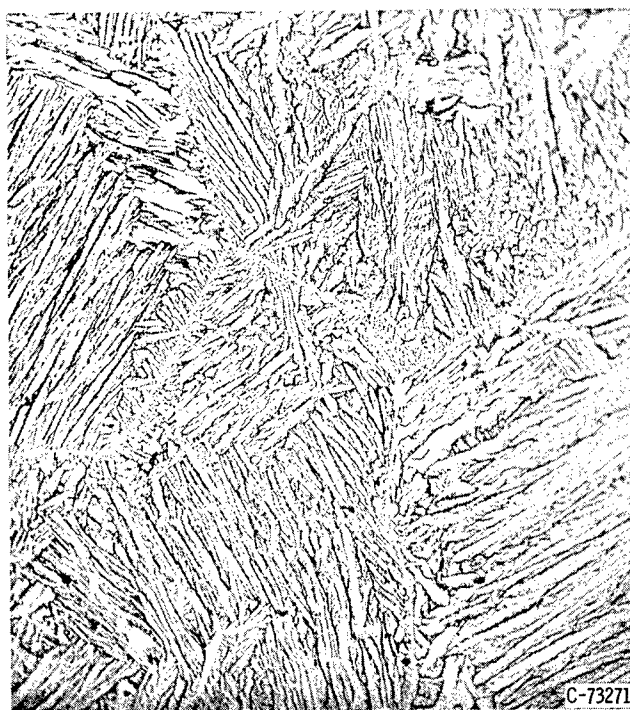
Figure 3. - Microstructure of sample containing 74.8 atomic percent vanadium. Primary phase, V_3Ga (white); secondary phase, V_6Ga_5 . Etchant, 4H_2O-3HNO_3-1HF ; X250.
