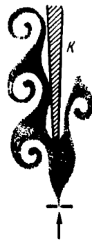
Figure 61. Vortexes in an organ pipe; air containing smoke is blown through the pipe
