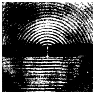
Figure 31. Aperture smaller than the wave length. The aperture becomes a source of waves spreading in semi-circles
