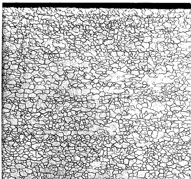
(a) 0.040-Inch-thick molybdenum specimen annealed at 2000° F in vacuum.
