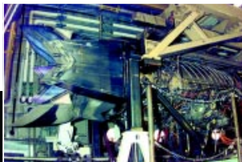
P&W F119 engine for F-22 Raptor in sea-level test cell SL-2
