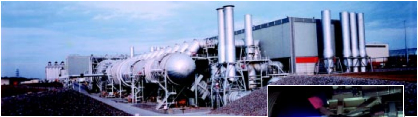
Aeropropulsion Systems Test Facility tests large turbofan commercial and military engines under simulated flight conditions.
