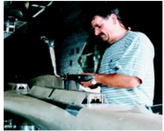
Weapons separation test on B1-B Lancer bomber
