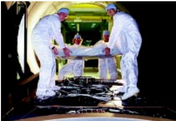
The mirror for the Far Infrared Submillimeter Telescope (FIRST) satellite program is shown being installed inside Space Environment Chamber 10V for testing.
