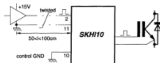
Fig.4b Connecting the SKHi10 with long cable
