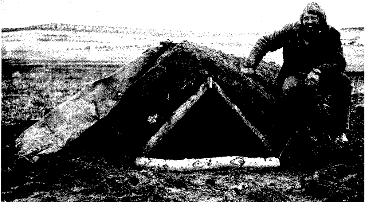
Figure 8.2 Half-Scale A-Frame Pole Shelter With the End Opposite Its Entryway Removed, After Withstanding about 16 psi Overpressure Effects.
