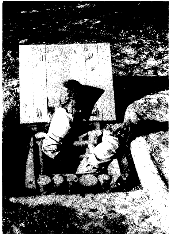
Figure 3.6 Photographer upside-down in Entryway of Half-Scale Small-Pole Shelter LN316-1A After the Blast. The fireball accompanying the 29 psi blast overpressure blackened the earth. The expedient blast door, the entryway, and the blast-protection frame of four notched-together logs were undamaged.
