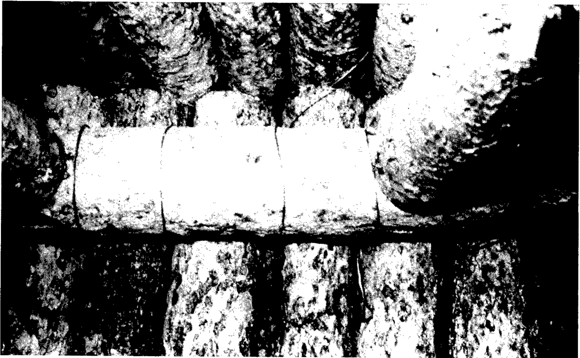
Figure 3.8 Detail of Small-Pole Shelter LN316-1B, showing wall poles, roof poles, longitudinal pole and two crossbraces after being subjected to 29 psi surface overpressure. Relative to bedrock, the whole shelter was permanently forced down 2-1/2 inches into the 2 feet of refilled earth on which it rested.
