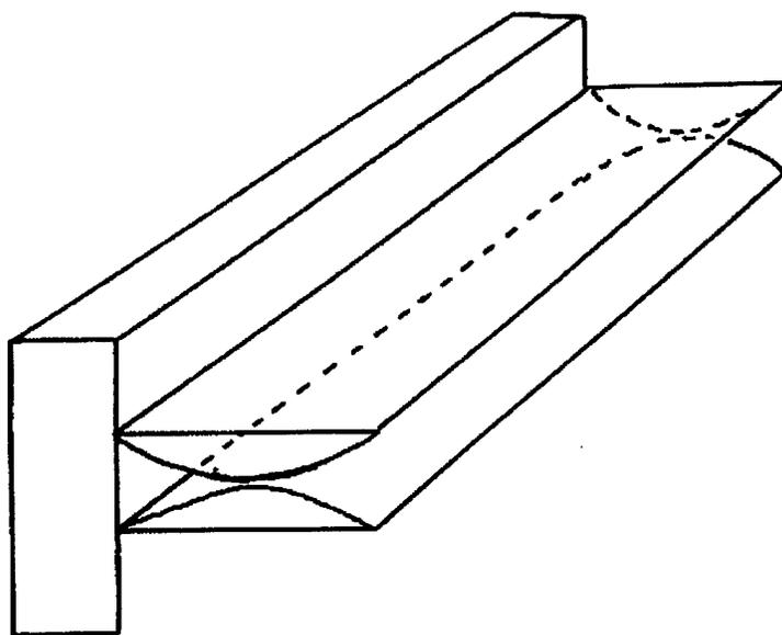
Figure 28. Schematic illustration of two flextensional cantilevers with contacts facing one another.
