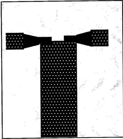
7. After Au/Cr is sputtered on the whole surface, another layer of SJR5740 photoresist is spin coated on the Au/Cr and patterned into transmission line by wet etch Au/Cr. Then the photoresist in the area of the transmission pad is exposed again.
