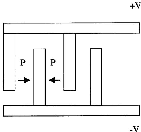
positive, when  $V > 0$  ( $E$  parallel to  $P$ ), the PZT will expand and the cantilever will bend downwards. When  $V < 0$  ( $E$  antiparallel to  $P$ ), the PZT will contract, and the cantilever will bend upwards.
