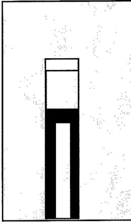
4. PZT at the end of cantilever is wet etched in HF and Pt/Ta below the PZT is etched by ion milling. Then the contacted bottom Au/Cr is formed on the appeared  $\text{Si}_3\text{N}_4$  by lift-off.
