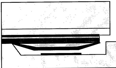
5. The glass wafer and the PZT coated silicon wafer are aligned and bonded together as shown.
