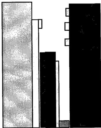
7. Finally, the silicon is etched by Deep Reactive Ion Etching (DRIE).
