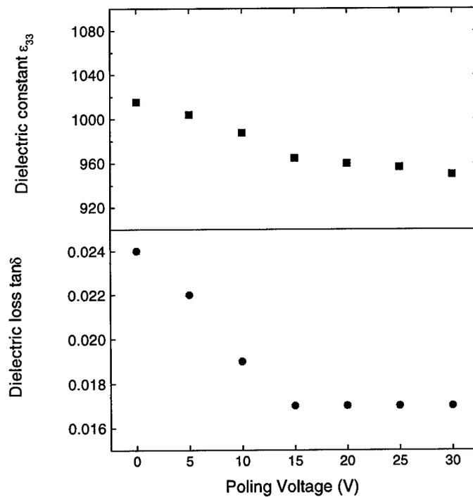
Figure 7. Dielectric constant and loss tan of the PZT film measured at a frequency of 1 kHz.
