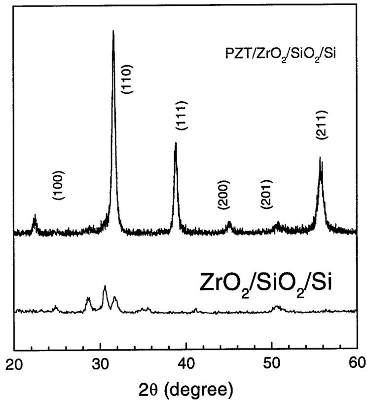
Figure 8. Pure perovskite phase was observed in the PZT film, and the structure was random without orientation.
