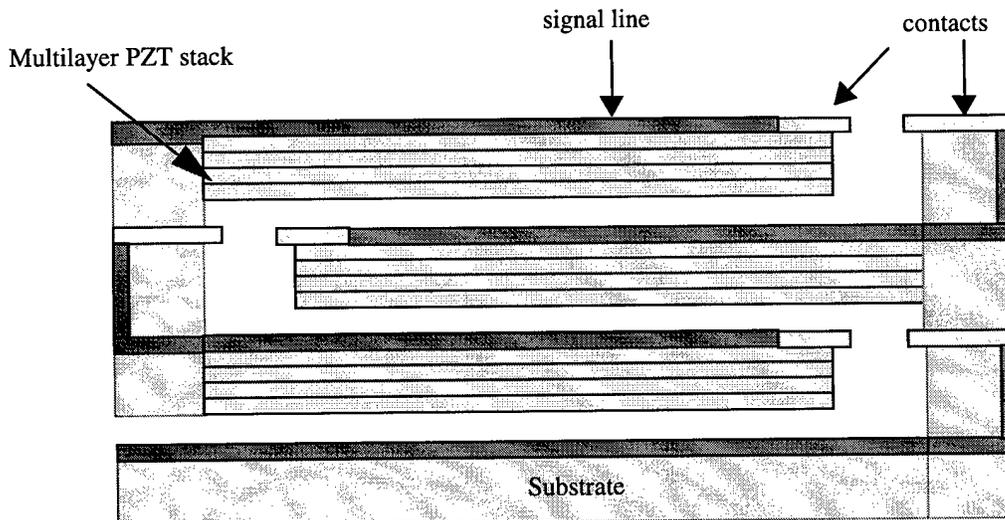
Figure 24. Series switch with stacked PZT layers
