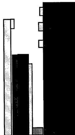
The PZT/ZrO<sub>2</sub> was patterned into a cantilever using ion milling, and the photoresist was subsequently removed with an O<sub>2</sub> plasma. The PZT/ZrO<sub>2</sub> is subsequently encapsulated with photoresist (1827), and RIE is used to pattern the Si<sub>3</sub>N<sub>4</sub>. The cantilever is released by etching the LTO in HF.
