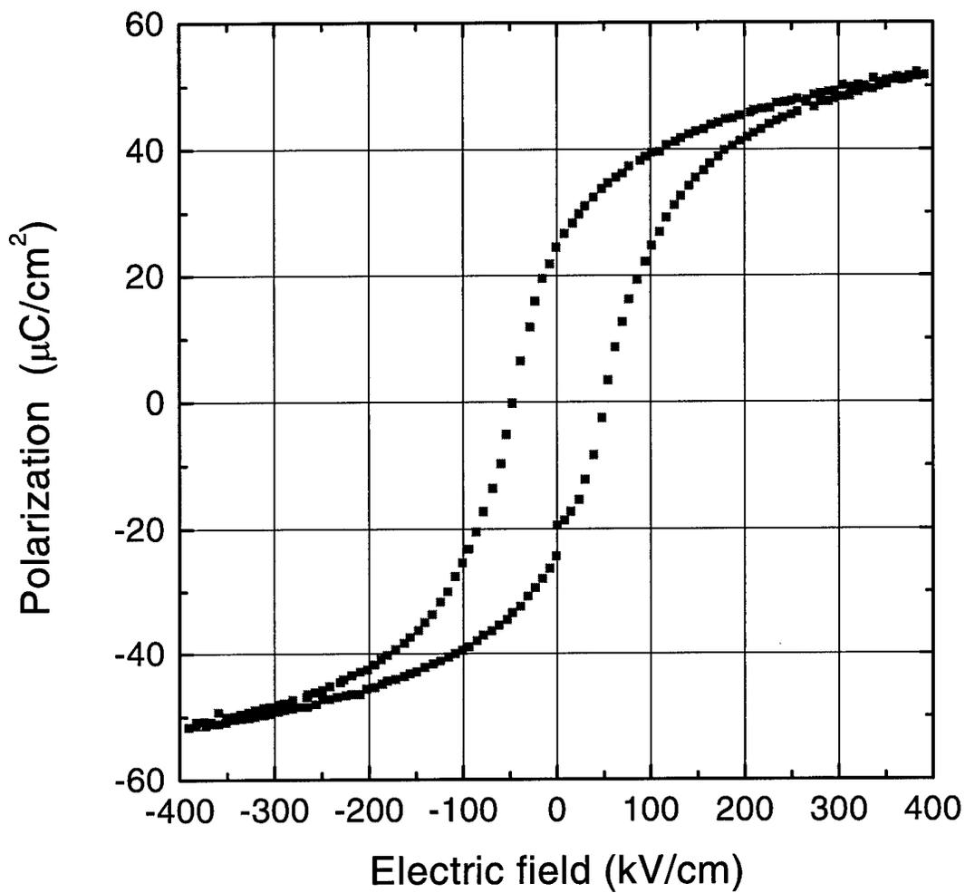
Figure 5. Polarization-Electric Field Hysteresis Loop measured with a RT66A ferroelectric tester. The remnant polarization and coercive field were  $25 \text{ C}/\text{cm}^2$  and  $46 \text{ kV}/\text{cm}$ , respectively.
