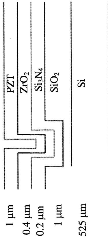
Figure 11. Samples of PZT film on ZrO<sub>2</sub>/Si<sub>3</sub>N<sub>4</sub>/SiO<sub>2</sub>/Si with anchors formed by etching away part of the SiO<sub>2</sub>.
