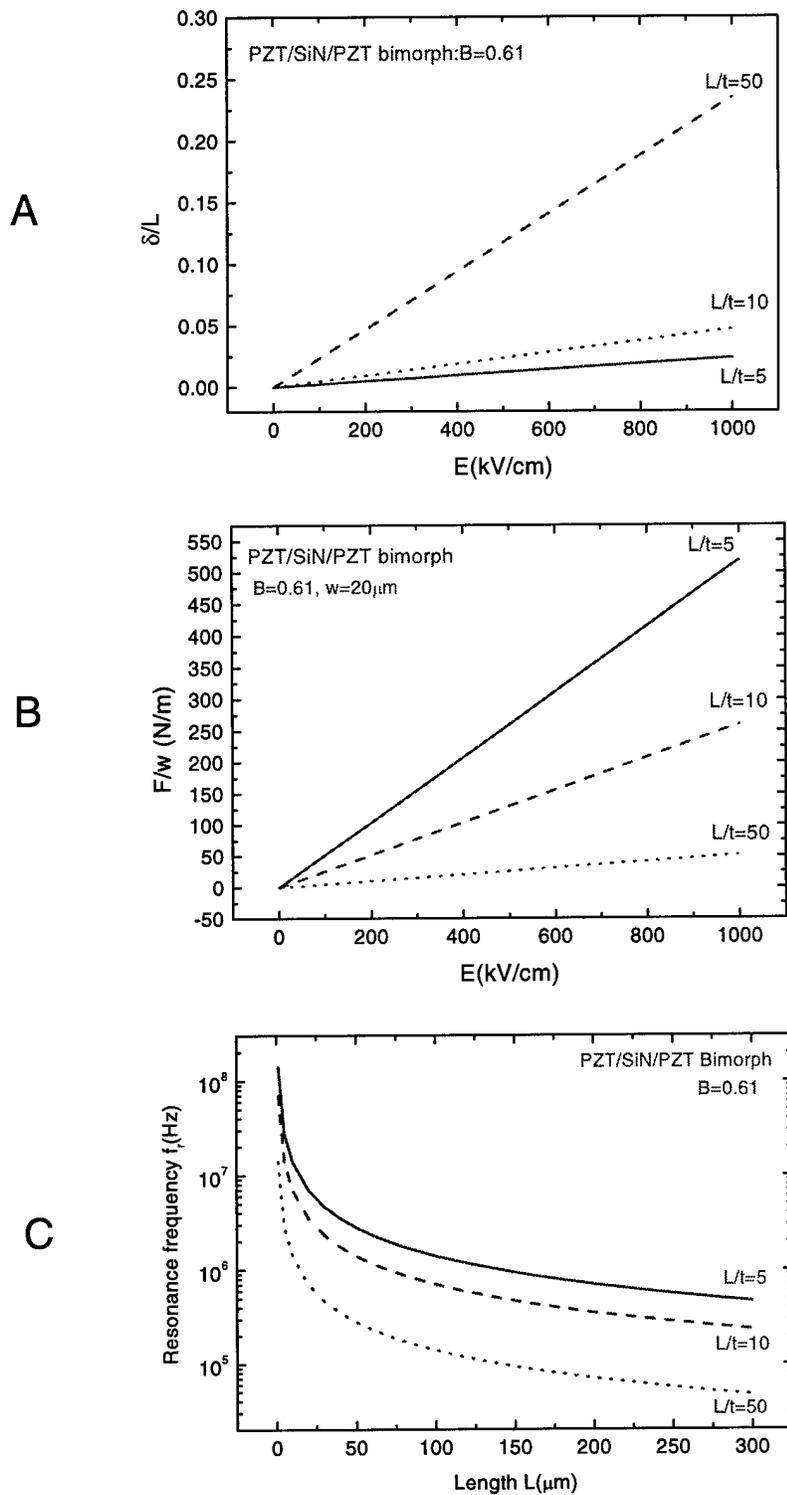
Figure 21. Calculated results for a bimorph arrangement. (a) Displacement expressed in units of cantilever length versus  $d_{31}$  electric field, (b) blocking force per unit width versus  $d_{31}$  electric field, (c) resonance frequency versus cantilever length for three length-to-thickness ( $L/t$ ) ratios.
