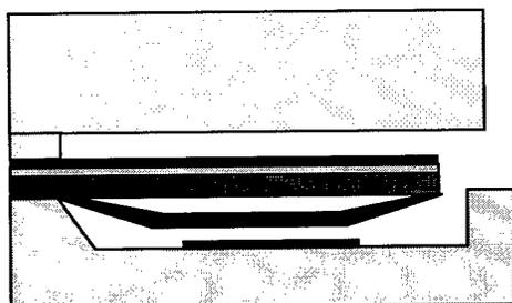
6. The sacrificial glass layer is etched under the PZT cantilever in HF. By controlling the aspect ratio of the structure, one can ensure that the cantilever is freestanding while the anchors are not etched away. Finally the polysilicon layer is dry etched in  $\text{XeF}_2$  dry etchant so as to release the flextensional gold structure.
