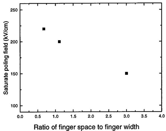
Figure 15. Dependence of current collected with interdigitated test electrodes versus poling electric field (upper panels and bottom left panel) and the saturation poling field versus the ratio of finger space to finger width,  $R$  (bottom, right panel).
