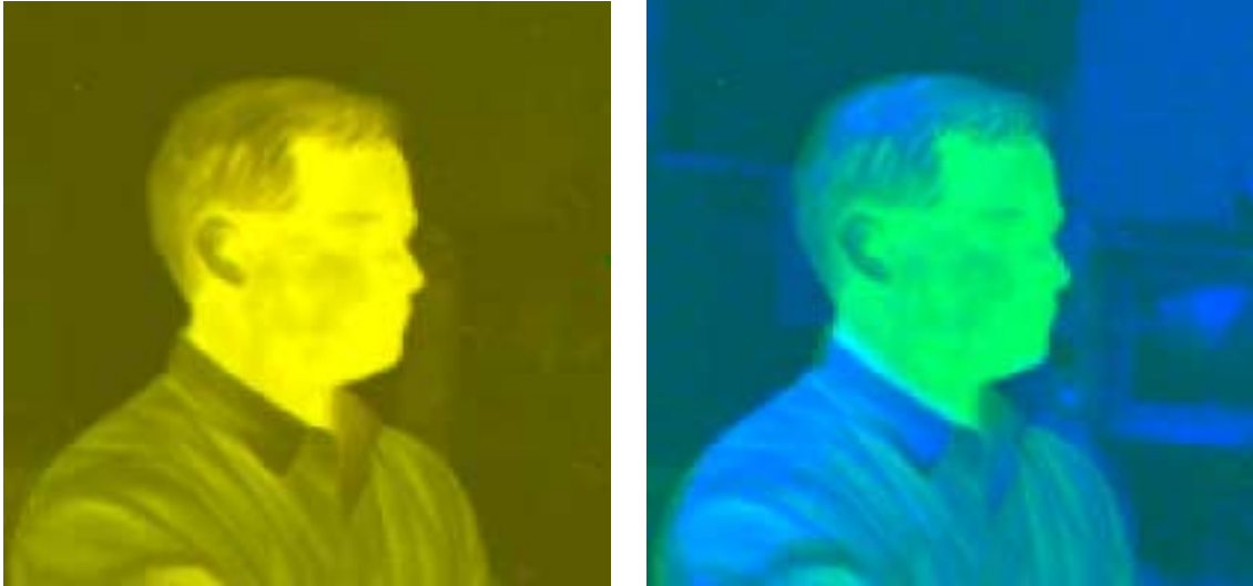
Figure 4. The system allows combination of bands to be compared. The left image is a two-color fused image of the two midwave bands, red and green. The data in the two bands is very similar and the person appears as a combination of red and green, yellow. The right image is a 2-color fusion of the shorter of the two midwave bands and the visible bands, green and blue. Note the visible band has information about the background. The person's shirt is more reflective in the visible and his skin emits in the infrared band. These two color fusion images were made by disabling the blue or red band in the 3-color Simple Fusion method and not with the 2-color color-opponency method.
