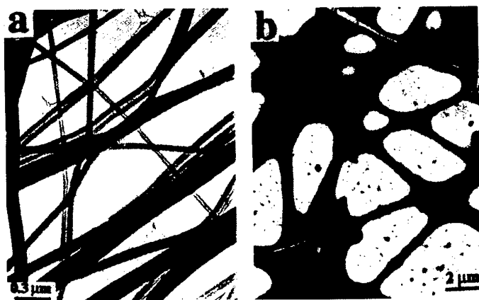
Fig 15. Tubules formed from a mixed-chain fluorocarbon/hydrocarbon glucophospholipid 22 as observed by cryo-transmission electron microscopy (a) (note the internal aqueous core) (from [96]), and by negative staining (b) (from [99]).
