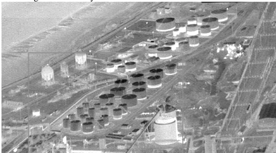
Figure 14. Nighttime MWIR image illustrating thermal signatures of fuel storage tanks. Unclassified Crown Copyright.
