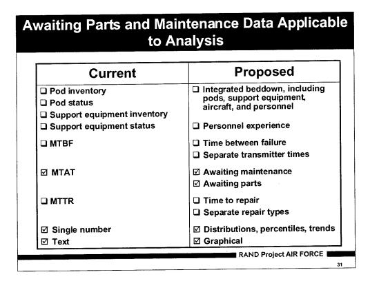
Currently, one can retrieve only base-level MTAT for a repair (the total time a pod spends from entry to exit of the repair shop) and MTTR (the time spent servicing the pod). By subtracting MTTR from MTAT, we can estimate the time awaiting maintenance or parts and shipment out of the shop. This data is available only for 184 long and short pods. Although this data can be used to compare wait times between bases, it is not specific enough to point to a particular problem.
