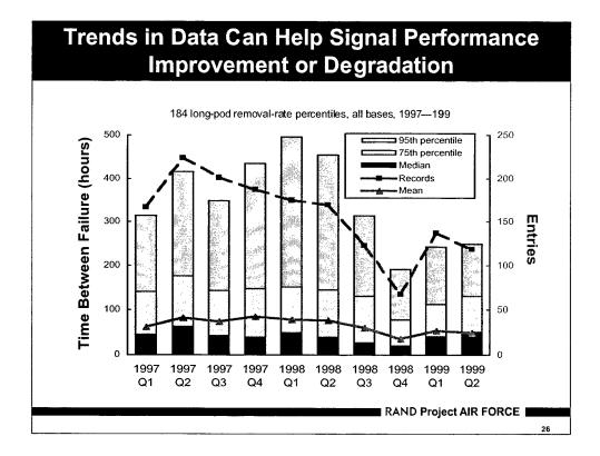
As mentioned earlier, a benefit of showing data over time is to signal possible developing problems with the pods. The chart above shows the percentiles of removal rates for 184 long pods between January 1997 and September 1999. This takes a similar look at the same data from the previous two charts but examines smaller time periods to see how the population of pod failures changes over time.
