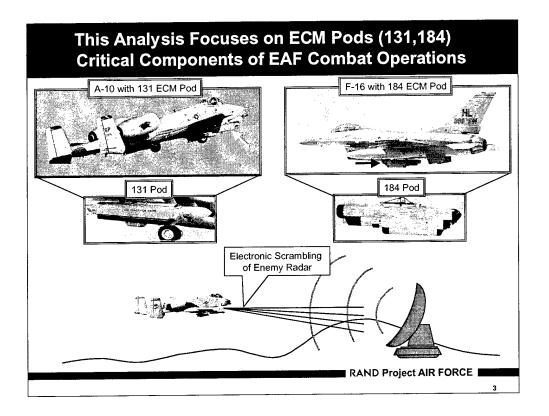
The ECM pod is a single pod mounted under the fuselage or wing of an aircraft. The pod allows for electronic scrambling of enemy radar, improving the survivability of engaged aircraft.
