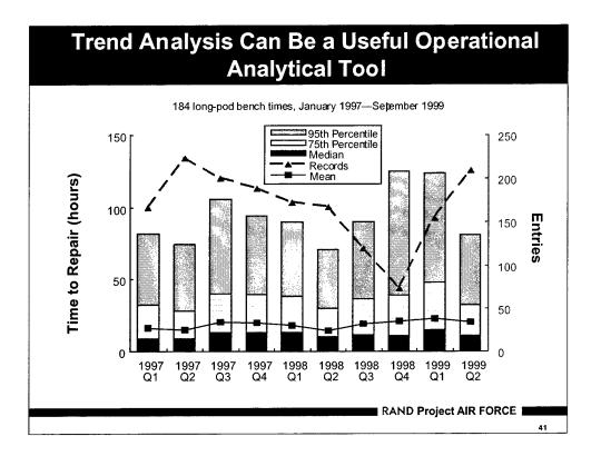
The chart above shows the monthly percentiles and averages of 184 longpod bench times between January 1997 and June 1999. Although the average time hovers around 20 hours, the median time (time below which half of all entries fell) is closer to 10 hours, and the rest of the entries were much higher than that. Again, the variation in the process can be seen with this type of data.
