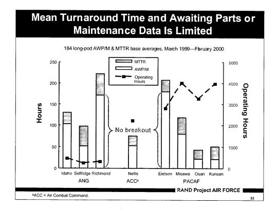
The chart above shows the awaiting parts and maintenance (AWP/M) time and MTTR for several bases for 184 long pods. Although there is variation in repair times, a significant proportion and variation of the MTAT is due to time AWM or AWP. Whether it is due to AWM or AWP is unclear from the available data. As described earlier, this wait time must be derived from two other summary statistics that are available on the RAMPOD web site.
