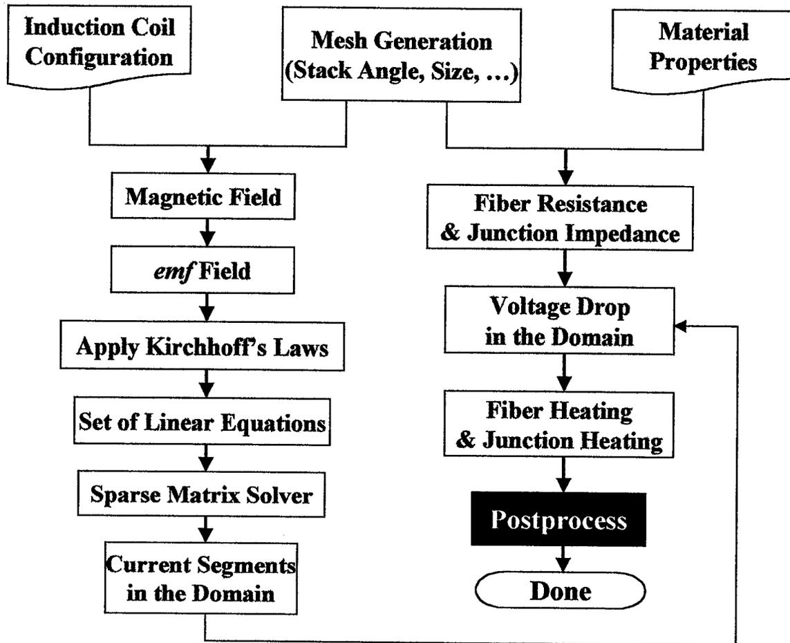
Figure 14. Schematic of a 2-ply heating model.
