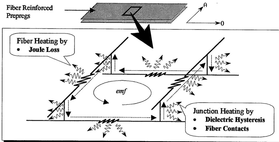
Figure 10. Heating mechanisms in each individual conductive loop.
