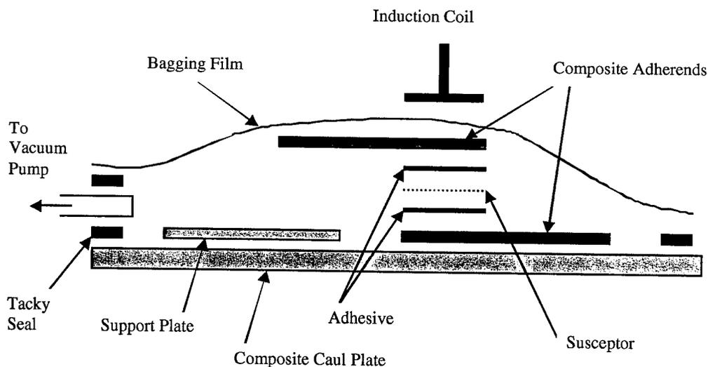
Figure 2. Specimen configuration during induction bonding.
