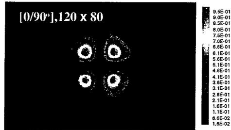
Figure 15. Comparison of heating patterns for [0/90] 2-ply stack.
