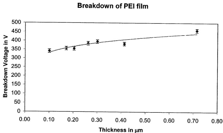
Figure 20. Breakdown voltage measurements for neat PEI films.
