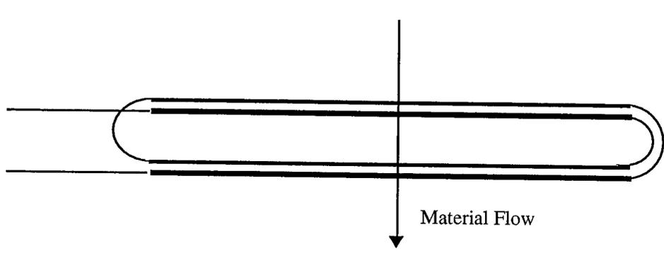
Figure 22. Schematic of rectangular coil for lamination stage.
