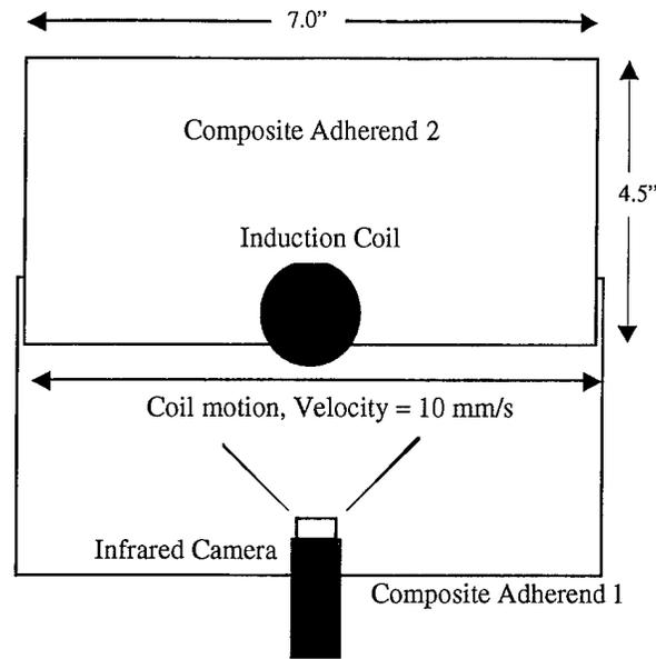
Figure 3. Induction coil motion direction and configuration.
