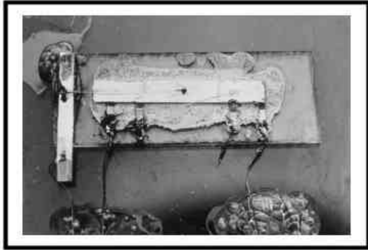
Figure 4. Jack Kilby's Integrated Circuit (Source: Texas Instruments, Inc.)
