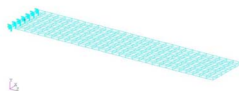
Figure 26. Patran Model Used to Determine Natural Frequencies.
