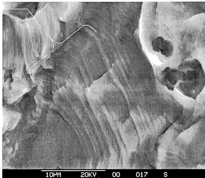
**Figure 87 Fatigue Striations from 15E20L, High Magnification**
