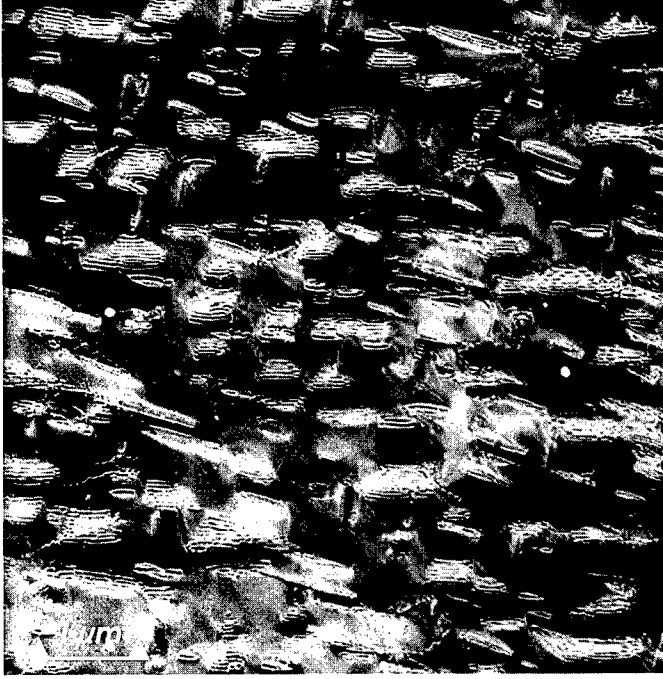
Figure 2. High-voltage transmission electron micrograph ( \sim 500 keV) showing large coherent precipitates of \text{Ni}_3\text{Al} in a Ni-13.53 at% Al alloy aged for 450 h at 700^\circ\text{C} .
