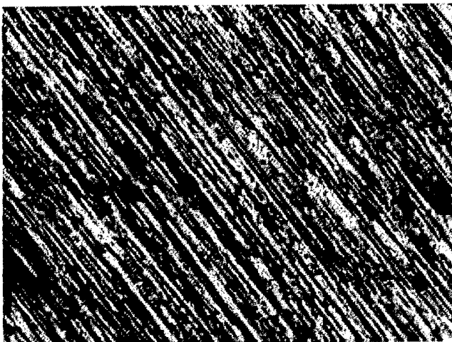
Figure 9 (a). AA2024-T3 before corrosion (1x 500).
