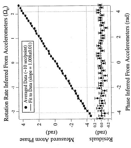
Rotation rate as inferred by the atomic interference pattern versus that measured directly using a pair of accelerometers.
