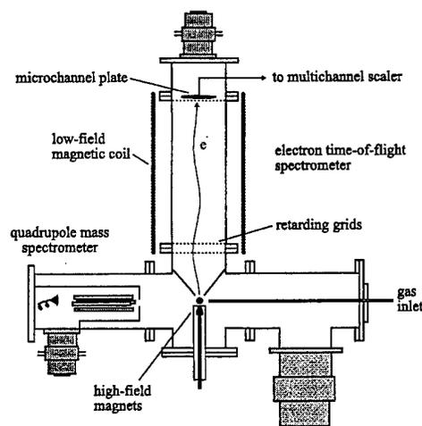
Figure 3. Detail of magnetic bottle time-of-flight electron spectrometer.
