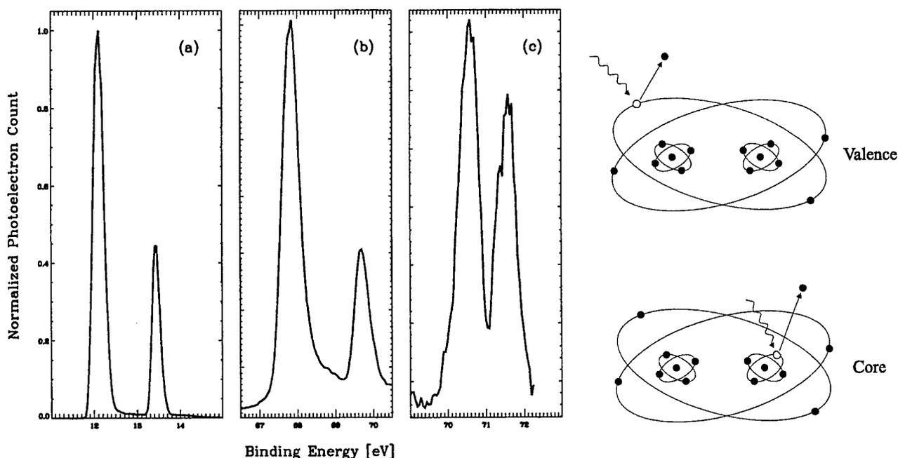
Figure 8. Spectrum of Xe and Br<sub>2</sub> with various harmonics. (a) Xe with the 11th harmonic, (b) Xe with the 47th harmonic, (c) Br<sub>2</sub> with the 49th harmonic. In the panel to the right is shown a schematic of the basic idea that the electrons arise from either valence shells, such as in (a) or inner shells, such as (b) and (c), depending on the photon energy.
