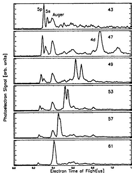
**Figure 4. Sample photoelectron spectra vs. arrival time for xenon with selected harmonics, 43rd to 61st, showing the 4d core electron features, the 5s and 5p valence electron peaks, and Auger transitions, which do not shift with photon energy. Acquisition of typical spectra requires only a few minutes of data collection.**
