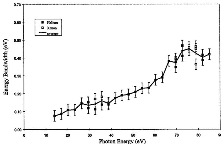
Figure 7. Measured bandwidths of individual harmonics. The symbols represent different species ionized. All experiments utilize the retarding grids.<sup>46</sup>
