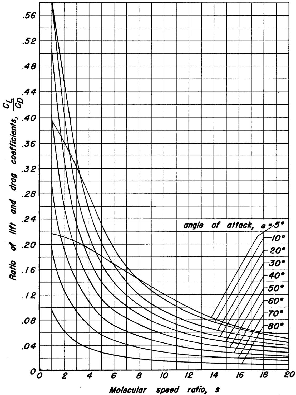
Figure 6.- Flat-plate lift-drag ratio, diffuse reflection.
