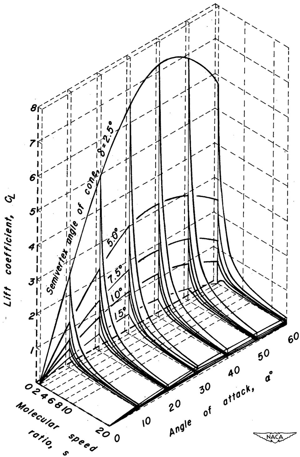
Figure 11.— Cone lift coefficient, diffuse reflection.
