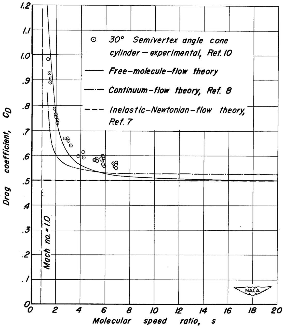
Figure 14.- Cone drag coefficient, comparison of free molecule and continuum-flow theory;  $\alpha = 0^\circ$
