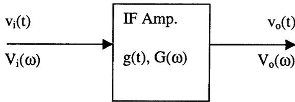
**Figure 3-1** Linear Swept Frequency Model
