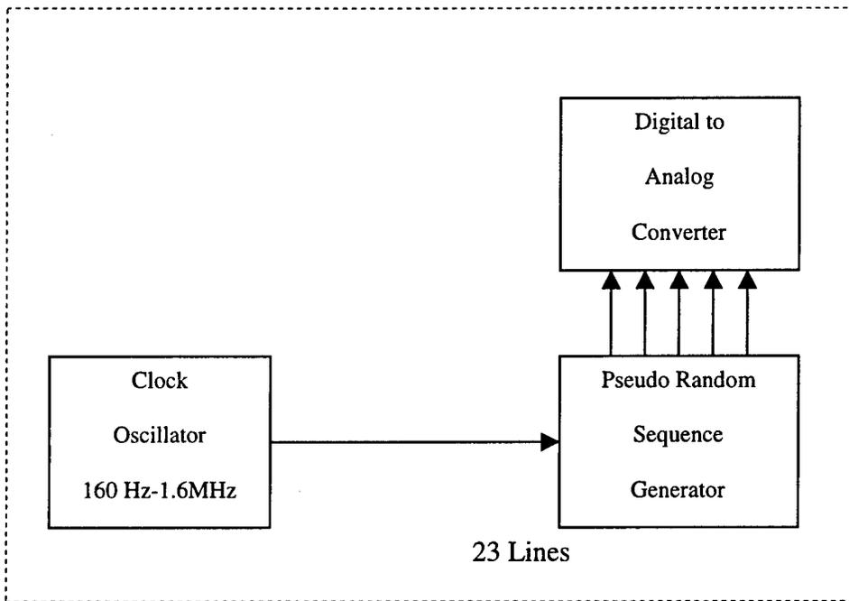
**Figure 4-2** Digital Filter of the Noise Generator
