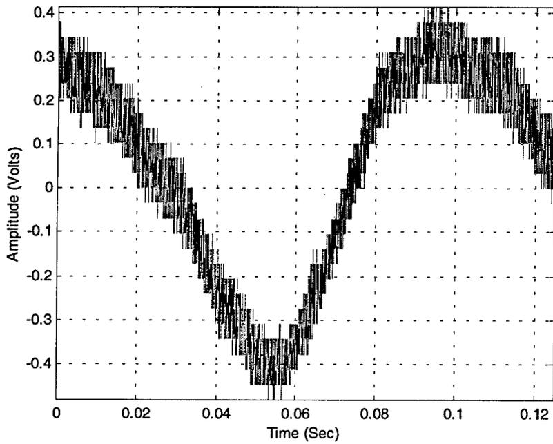
**Figure 4-5** 10 Hz Sinewave Noise Modulation, IF Bandwidth = 0.1 MHz
