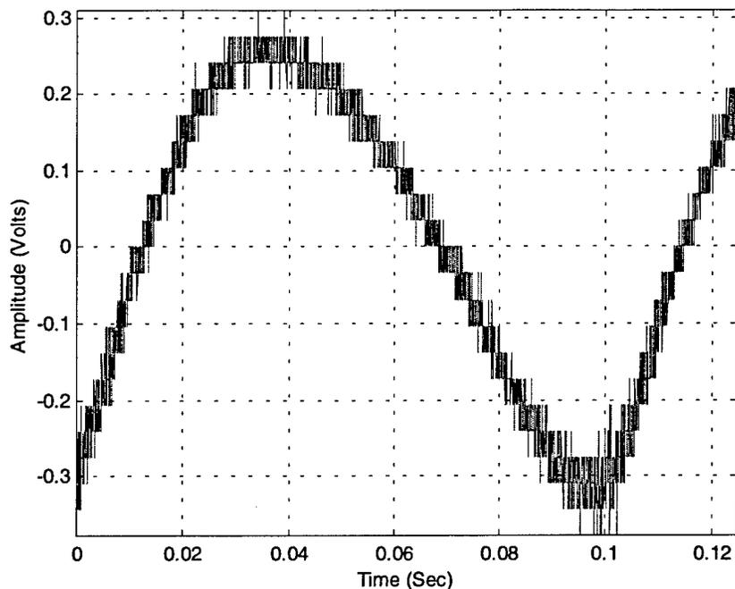
**Figure 4-8** 10 Hz Sinewave Noise Modulation, IF Bandwidth = 30 MHz
