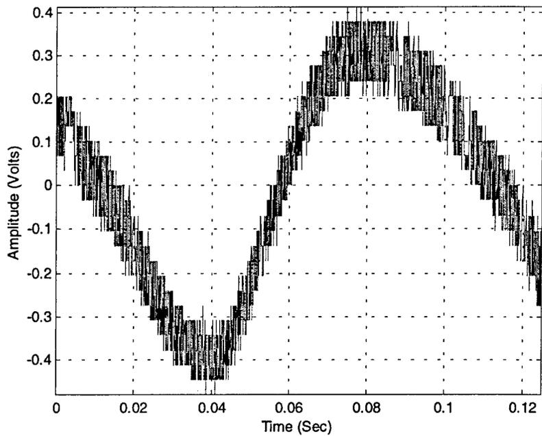
**Figure 4-6** 10 Hz Sinewave Noise Modulation, IF Bandwidth = 1.0 MHz
