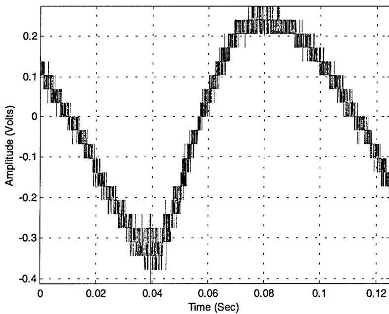
**Figure 4-7** 10 Hz Sinewave Noise Modulation, IF Bandwidth = 5.0 MHz
