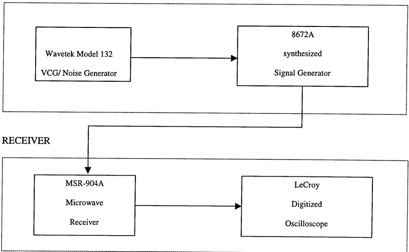
**Figure 4-1** Block Diagram of Equipment
