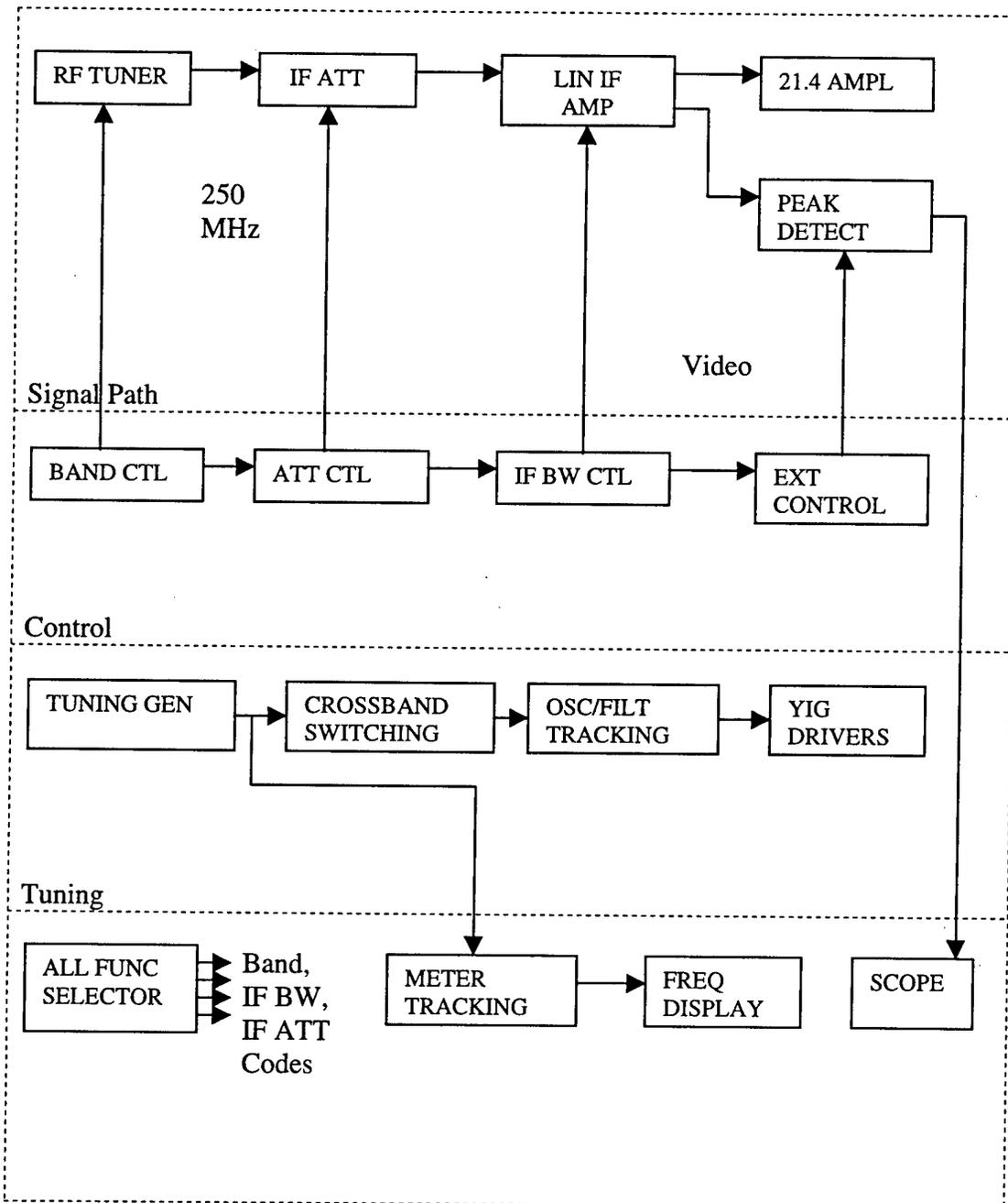
Figure 4-3 MSR-904A Block Diagram (1:5)
