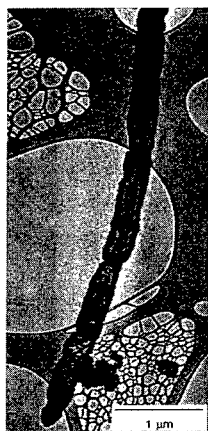
Fig.3 TEM: The worm-like material are chains of multi-walled carbon nanoparticles
