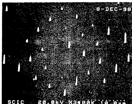
Figure 5B. Growth of single carbon nanotubes on each nickel dot spaced by 5 \mu\text{m} .
