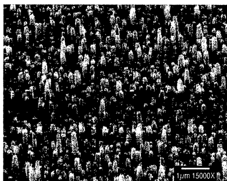
FIGURE 2B. SEM image of very short carbon nanotubes grown on silicon for only 2 minutes.
