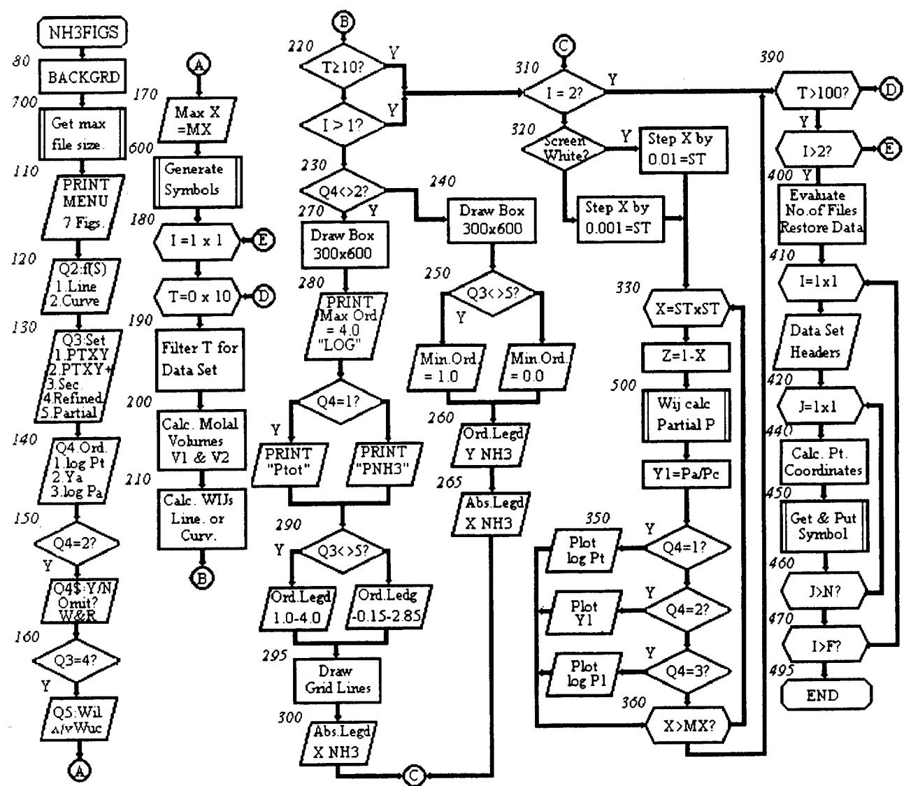
Figure 8. Flowchart for Graphical Comparison of  $W_{ij}$  Results
