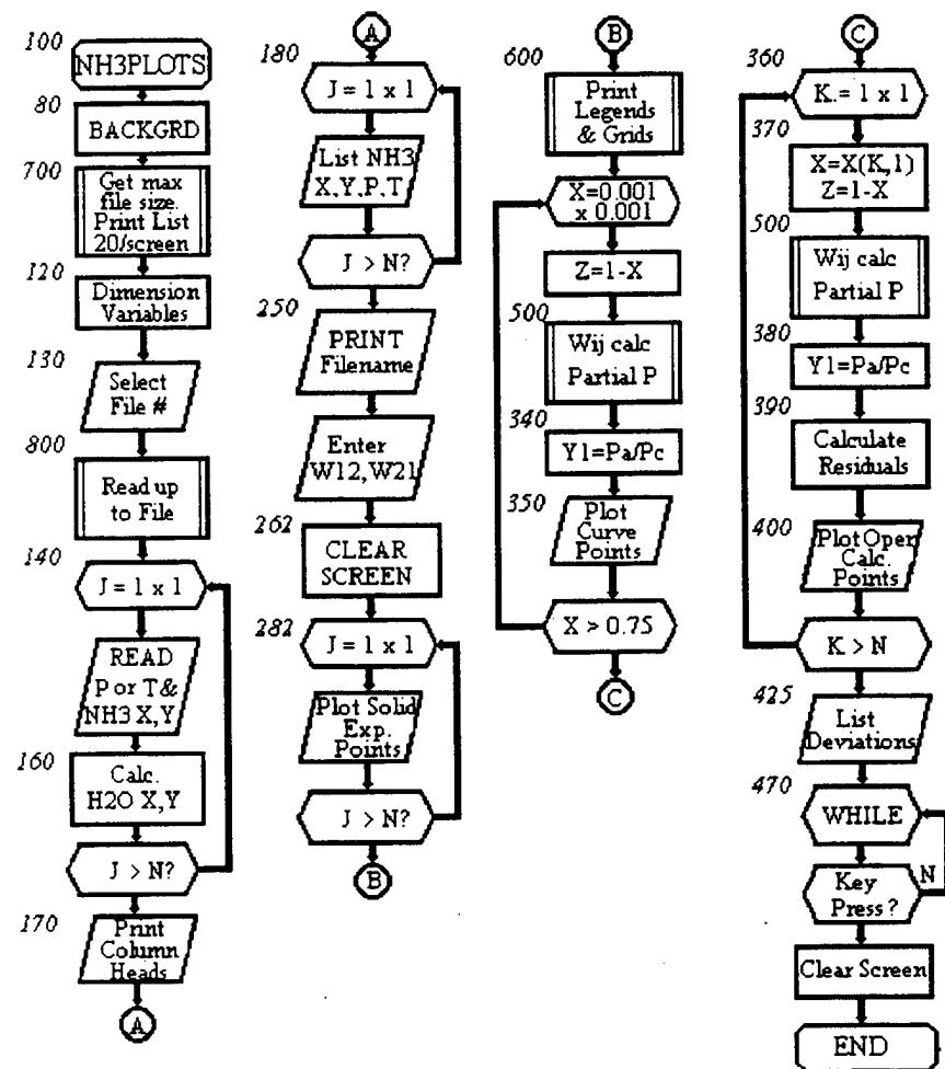
Figure 6. Flowchart for Graphing Vapor and Liquid Mole Fractions
