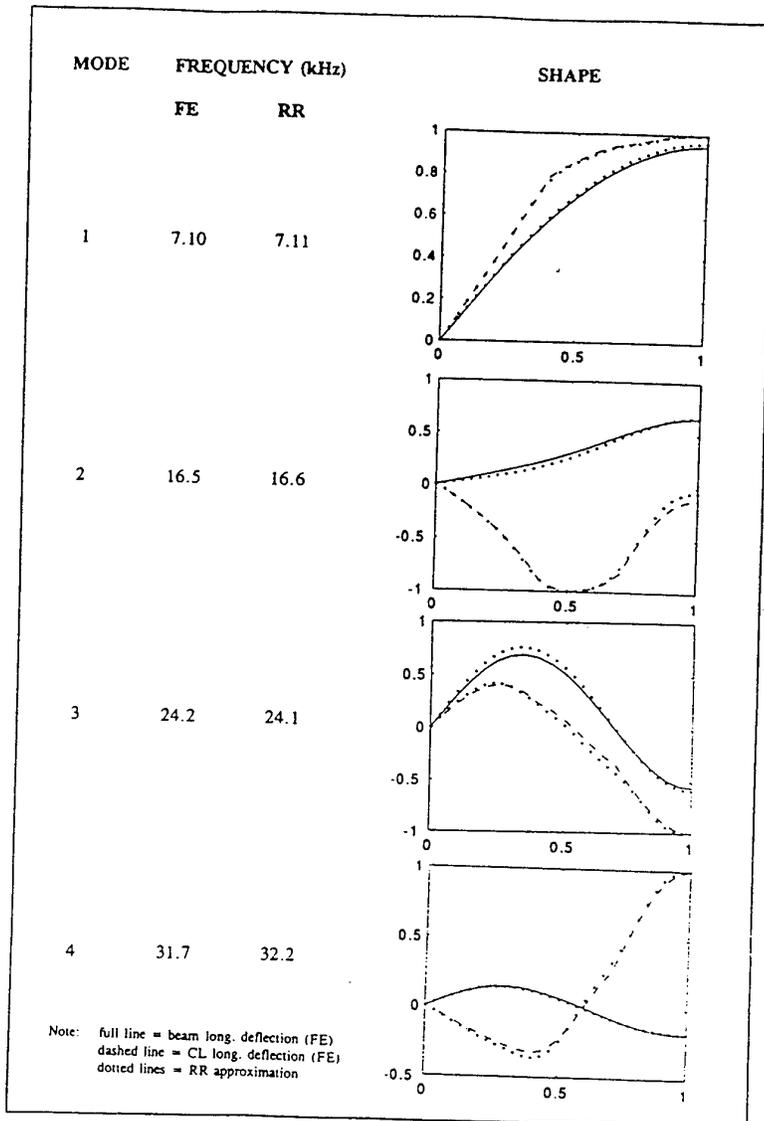
Fig. 8 Longitudinal natural frequencies and mode shapes
