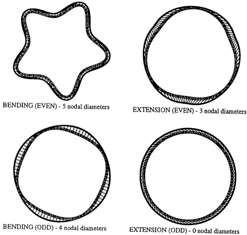
Figure 2. Constrained layer damped ring mode types.
