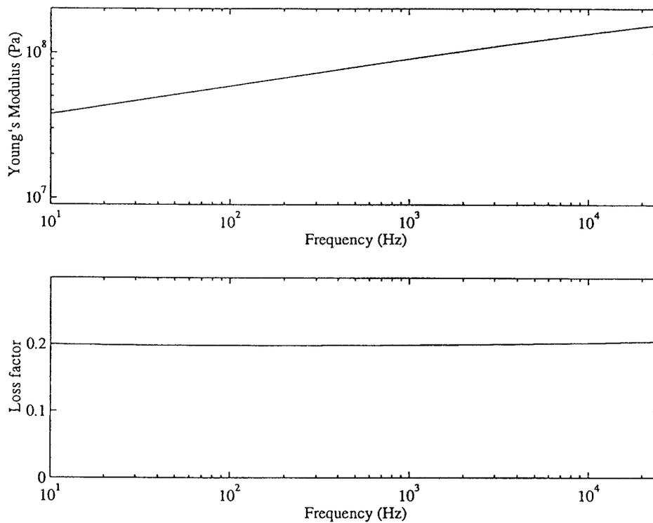
Figure 7. Material properties for polyurethane at 22°C.
