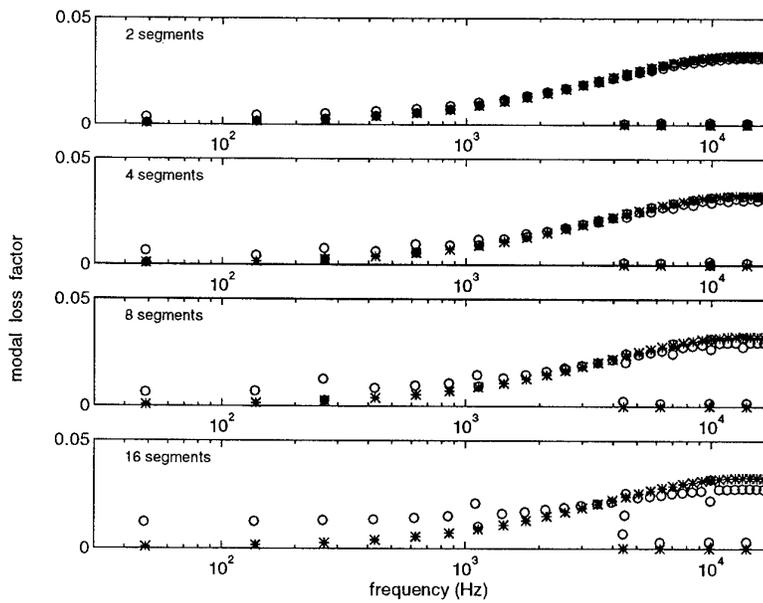
Figure 5: Loss factors of ring with segmented constraining layer  $E_v = 150$  MPa (\*\* unsegmented, oo segmented)
