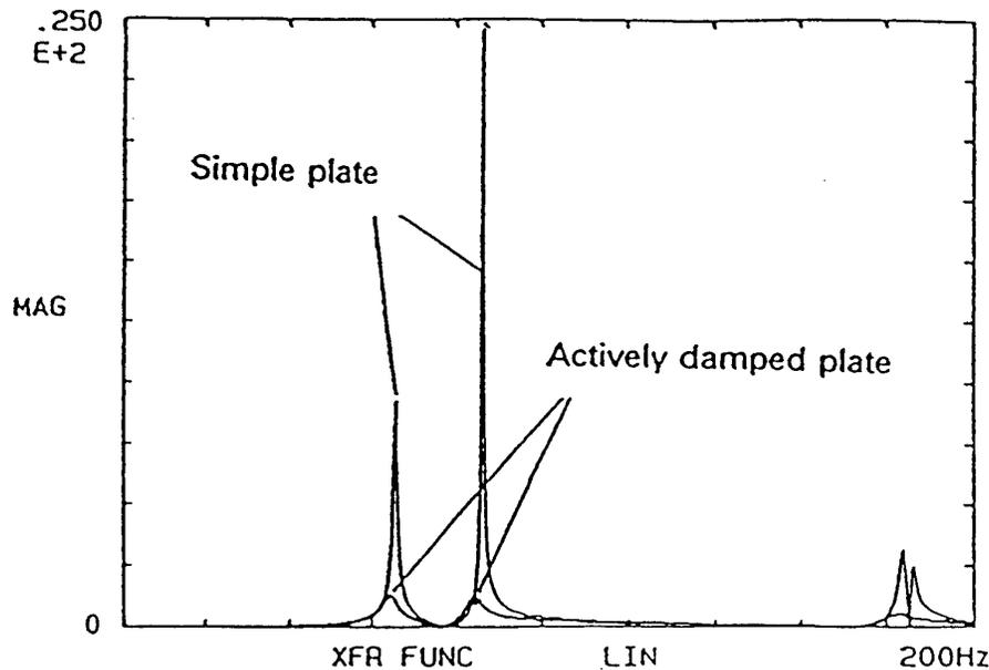
Figure 8 - Active Damping Applied to a plate structure
