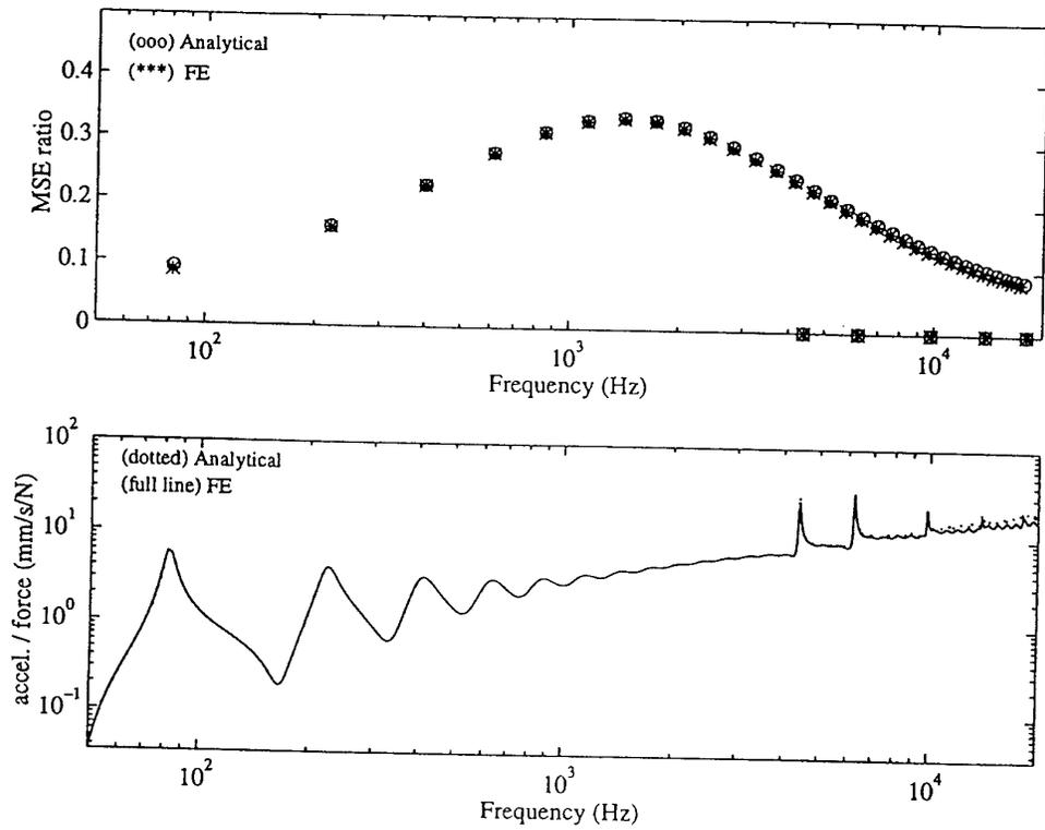
Figure 3. Comparison of analytical and FE results for ring A.
