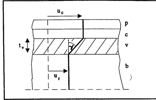
Fig. 3 Deformation of the beam in longitudinal motion
