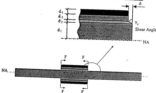
Figure 3. Local active damping with symmetrical actuators.
