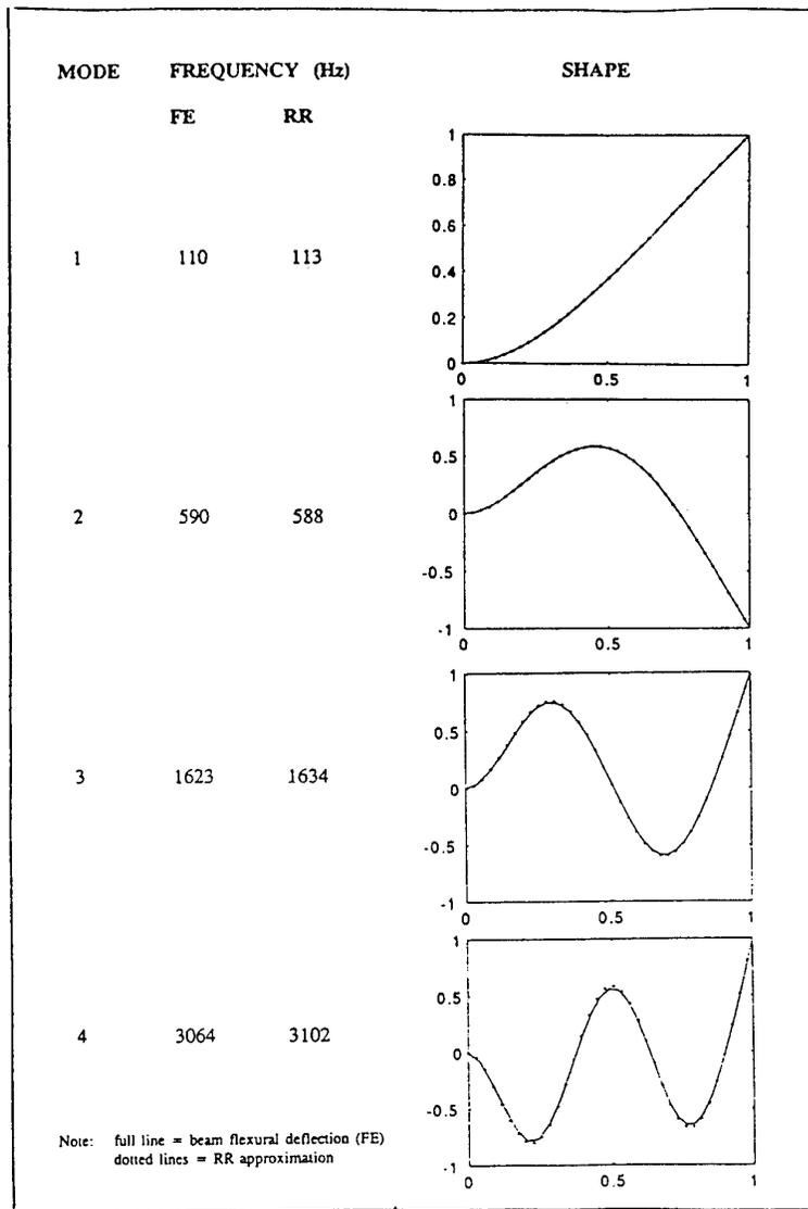
Fig. 9 Flexural natural frequencies and mode shapes
