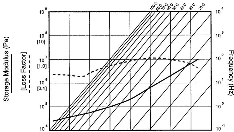
Figure 2: Shear modulus master curve for ISD 112
