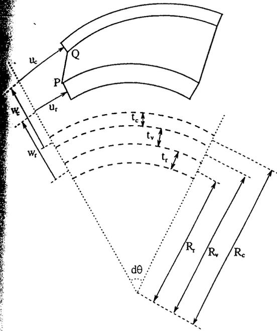
Figure 1. Deformation of a sandwich ring.
