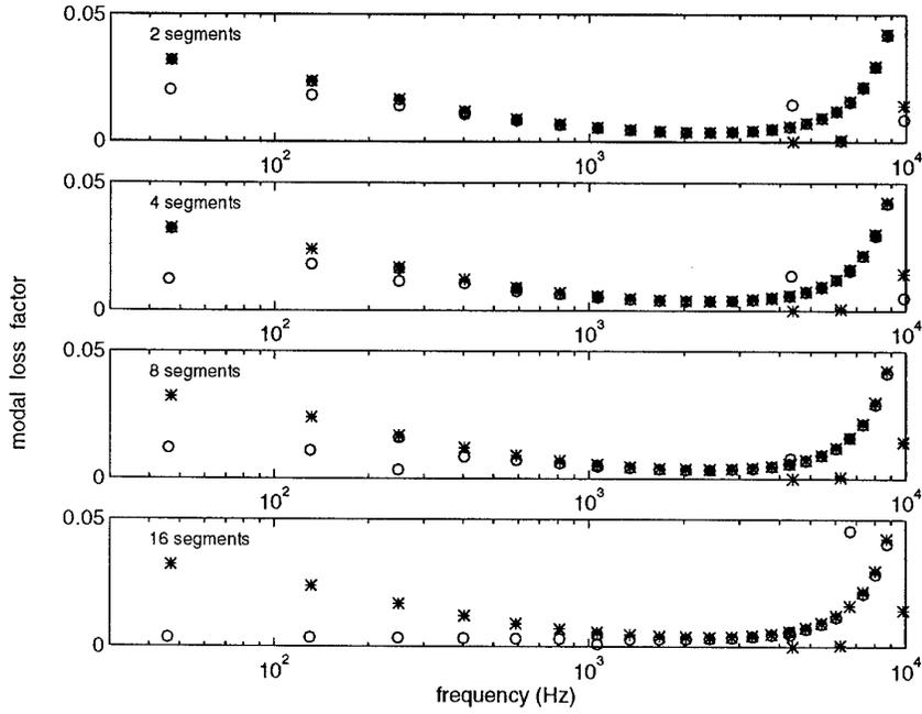
Figure 4: Loss factors of ring with segmented constraining layer  $E_v = 0.5$  MPa (\*\* unsegmented, oo segmented)
