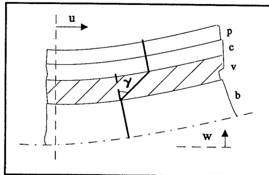
Fig. 4 Deformations of the beam in flexural motion
