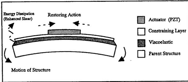
Fig. 1 "Active damping" concept—as defined in this paper
