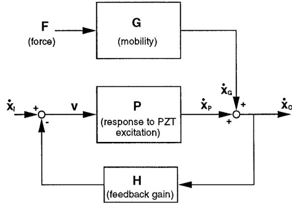
Figure 12: Schematic diagram of velocity feedback strategy
