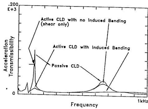
Figure 5. Active damping with and without bending moments.
