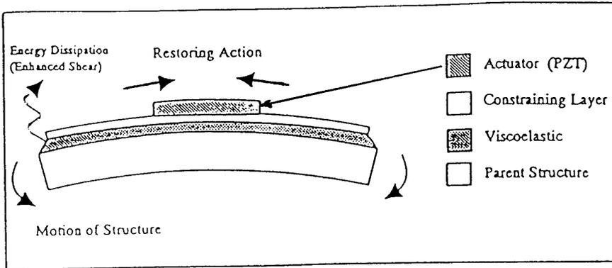
Figure 1 : Active Constrained Layer Damping (ACLD)
