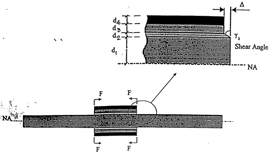
Figure 4 - Local Active Damping with Symmetrical Actuators
